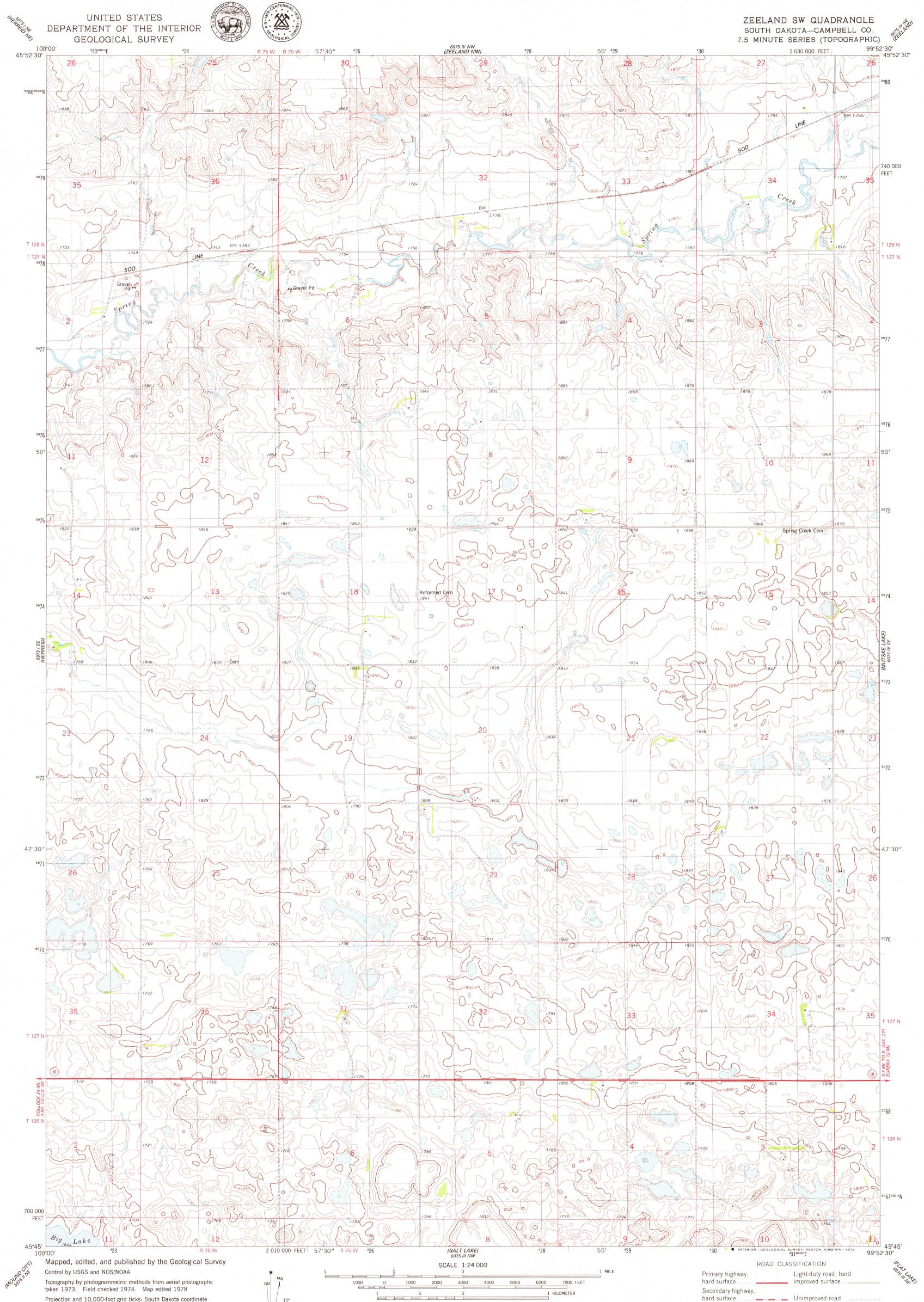
Projection and 10,000-foot grid ticks: South Dakota coordinate system, north zone (Lambert conformal conic) 1000-meter Universal Transverse Mercator grid, zone 14 1927 North American datum
