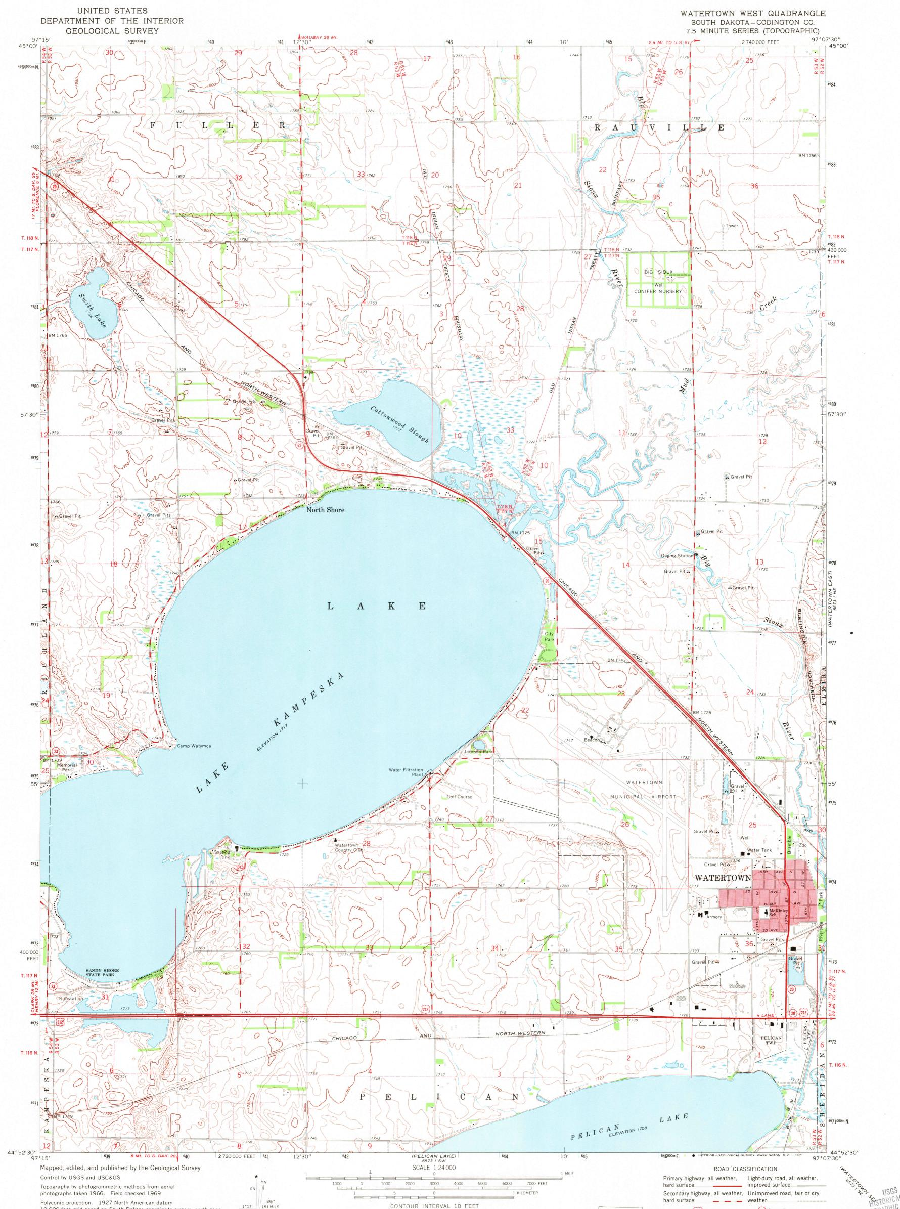
Polyconic projection. 1927 North American datum 1°17′ 23 MILS 10,000-foot grid based on South Dakota coordinate system, north zone 1000-meter Universal Transverse Mercator grid ticks, zone 14, shown in blue
