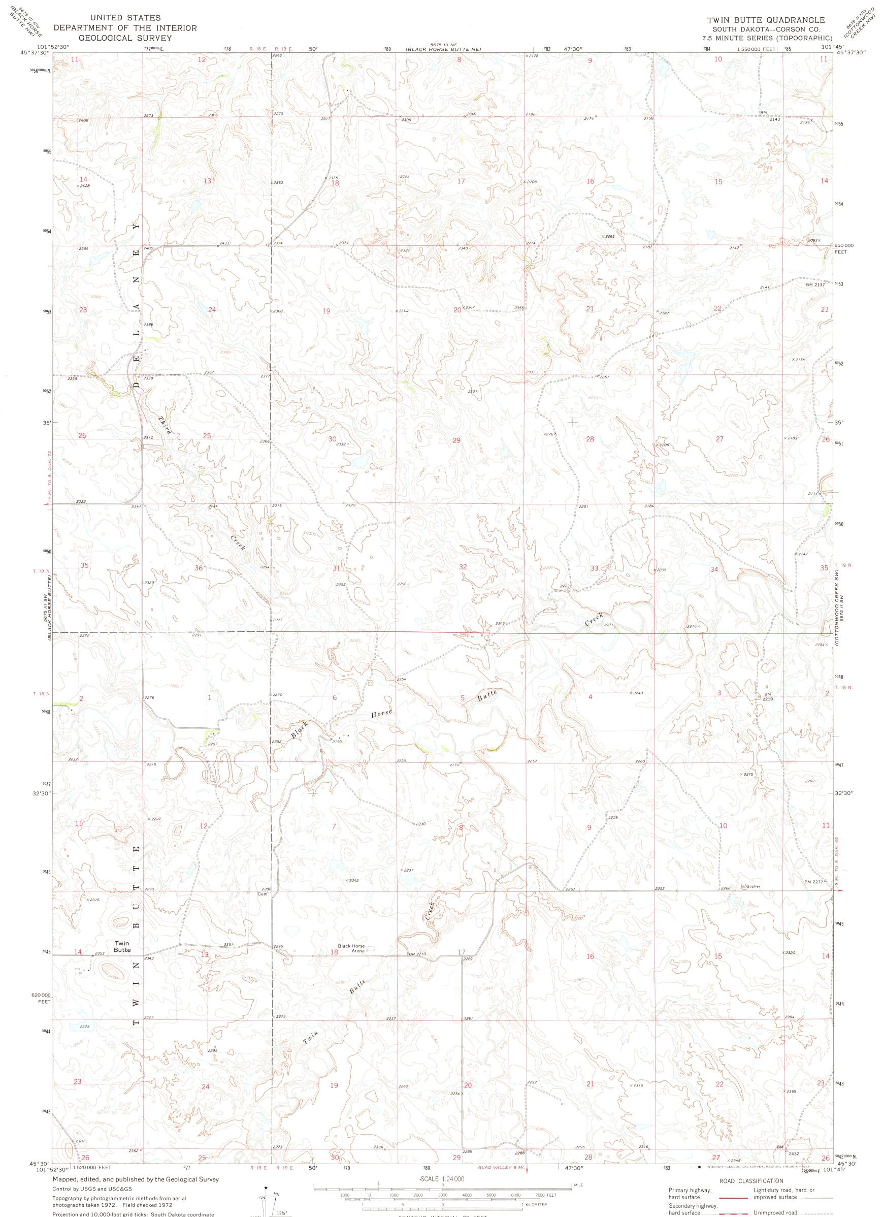
Projection and 10,000-foot grid ticks: South Dakota coordinate system, north zone (Lambert conformal conic) 1000-meter Universal Transverse Mercator grid ticks, zone 14, shown in blue. 1927 North American datum
