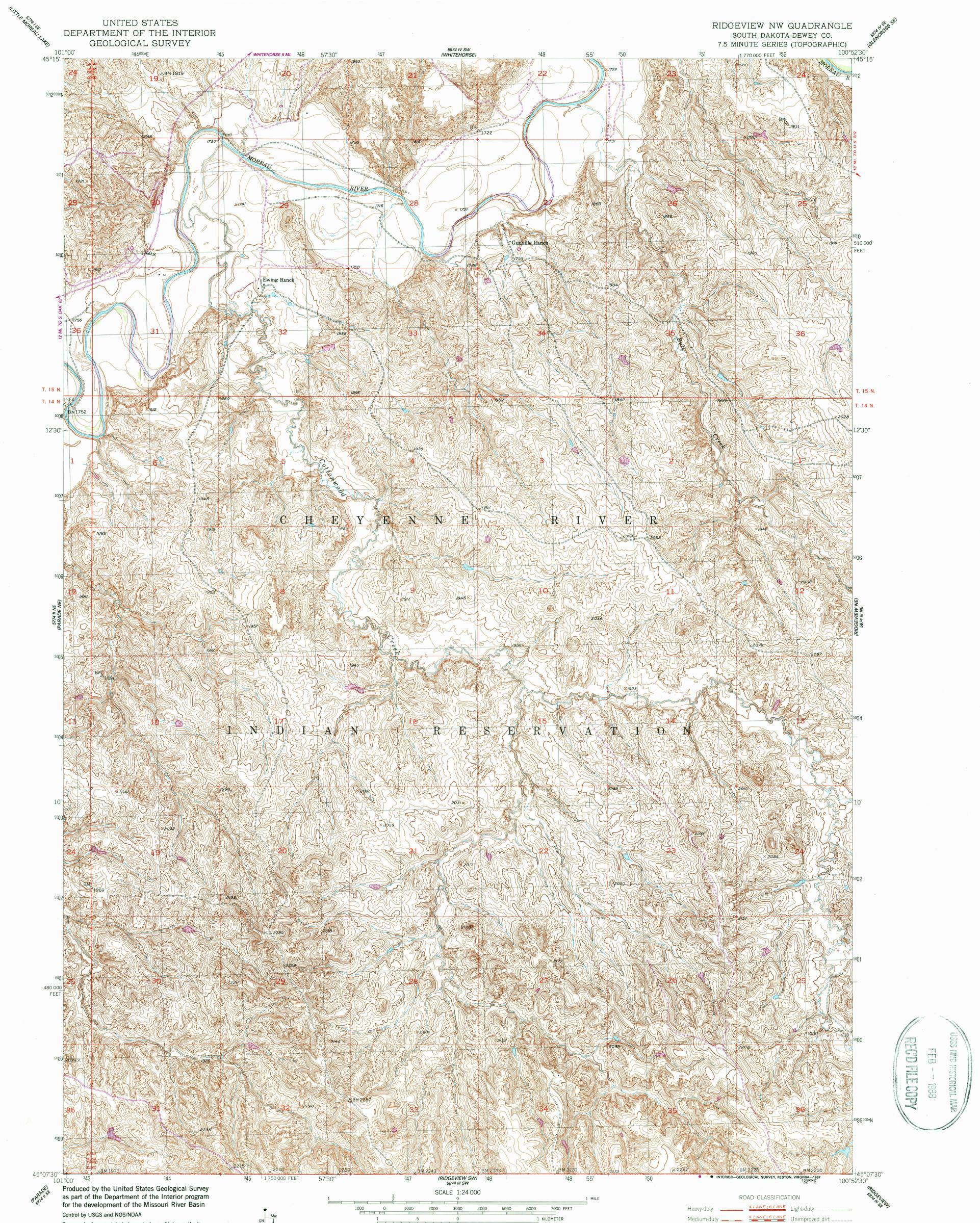
Topography from aerial photographs by multiplex methods Aerial photographs taken 1948. Field check 1951 Polyconic projection. 1927 North American Datum 10,000-foot grid ticks based on South Dakota coordinate system, north zone 1000-meter Universal Transverse Mercator grid, zone 14
