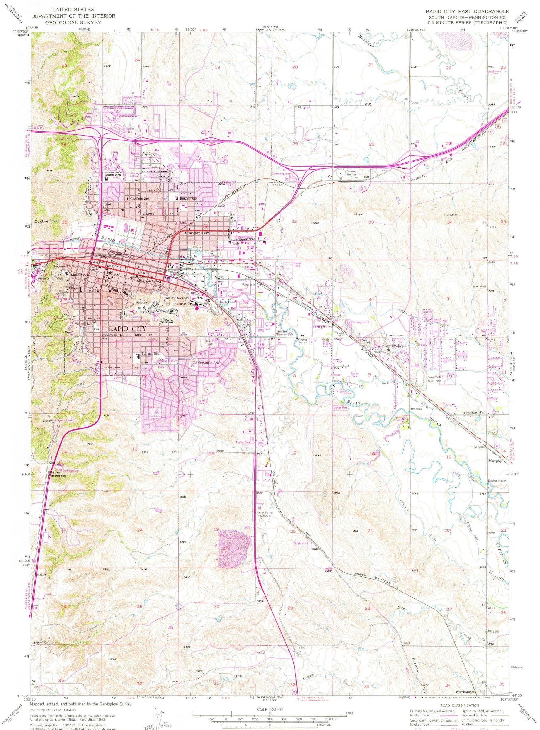
Polyconic projection. 1927 North American datum 10,000-foot grid based on South Dakota coordinate system, south zone Red tint indicates areas in which only landmark buildings are shown 1000-meter Universal Transverse Mercator grid ticks, zone 13, shown in blue Revisions shown in purple compiled from aerial photographs taken 1976 and other source data. This information not field checked. Map edited 1978 Purple tint indicates extension of urban areas
