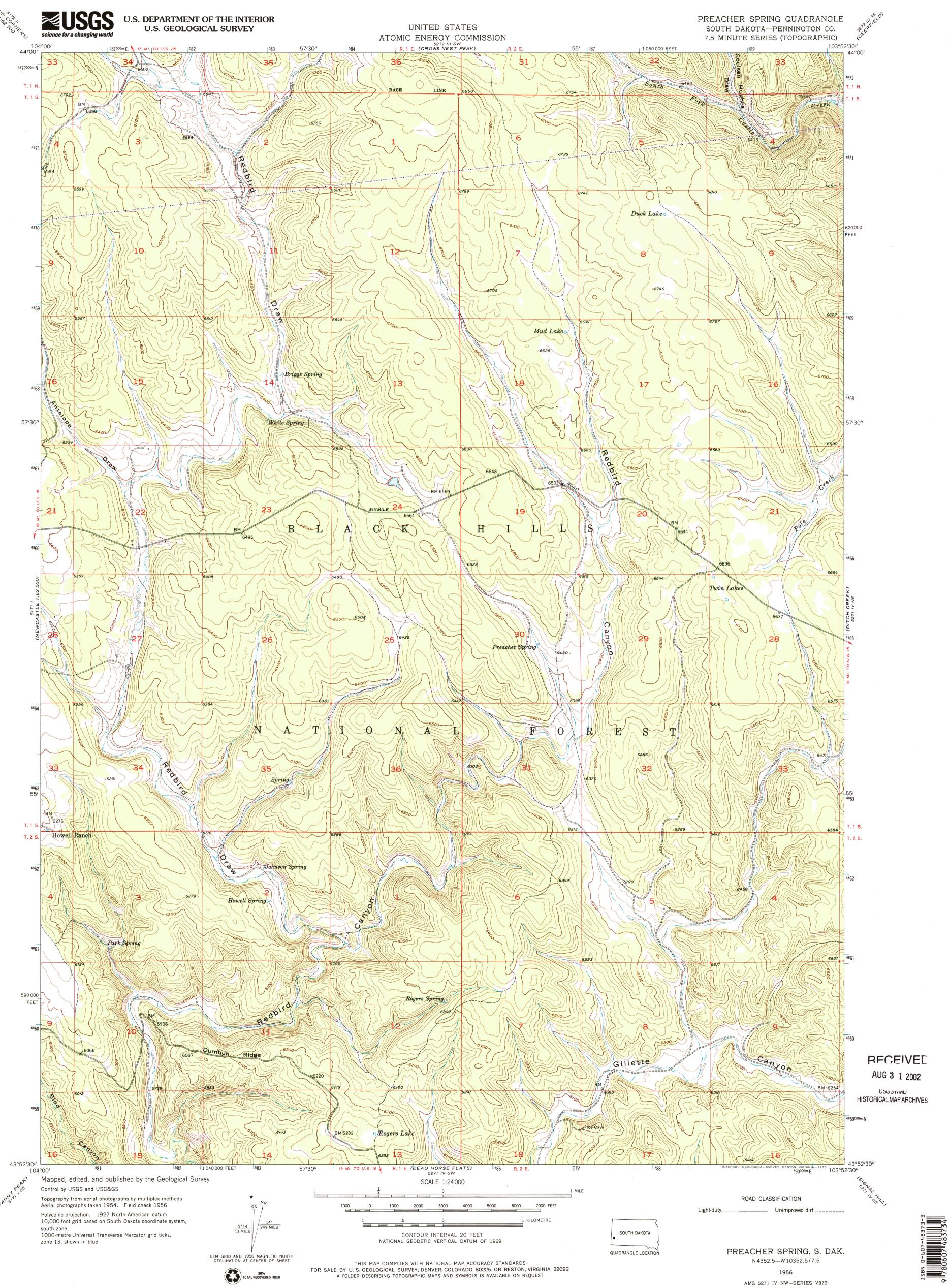
Polyconic projection. 1927 North American datum 10,000-foot grid based on South Dakota coordinate system, south zone 1000-metre Universal Transverse Mercator grid ticks, zone 13, shown in blue
