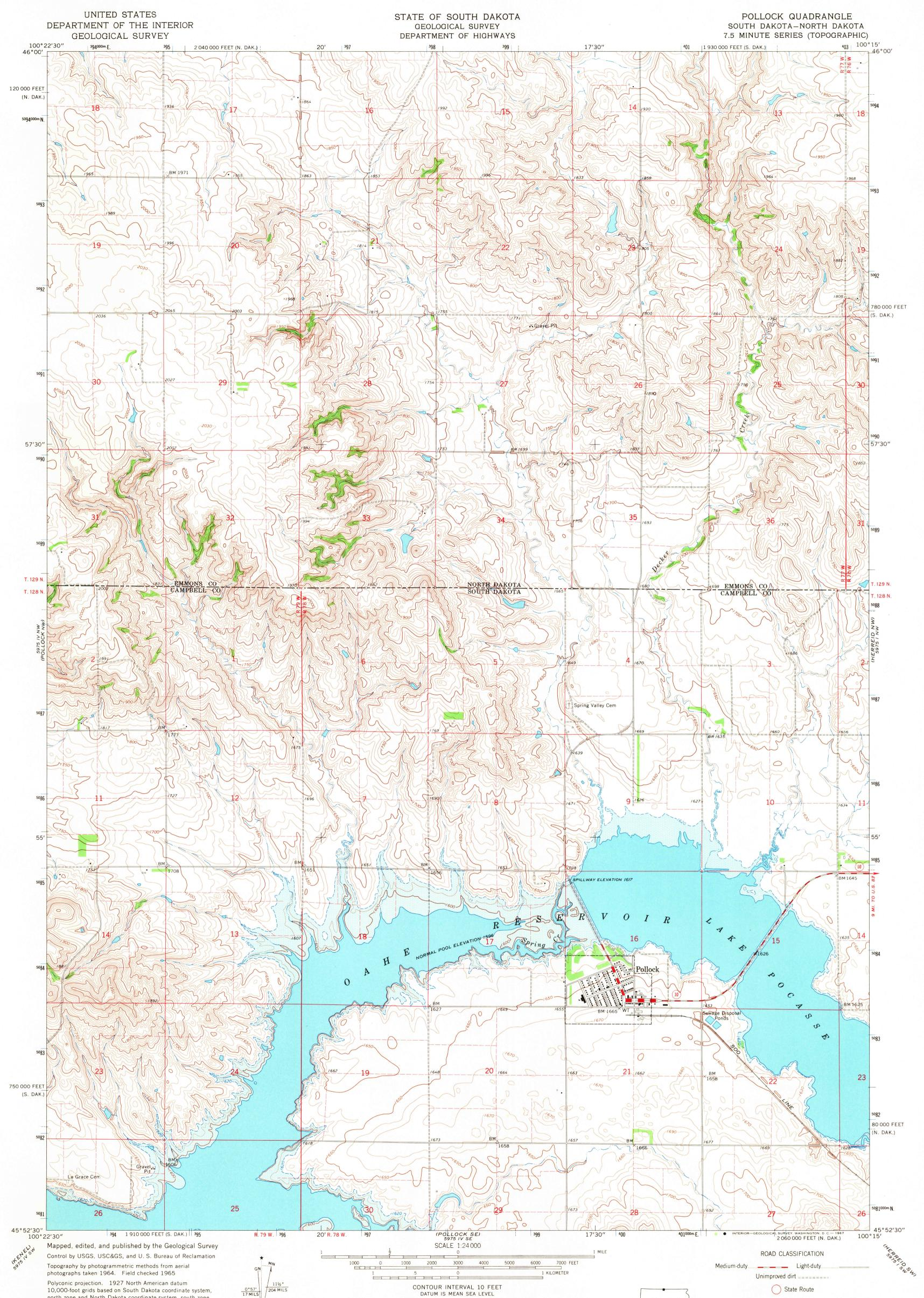
10,000-foot grids based on South Dakota coordinate system, north zone and North Dakota coordinate system, south zone 1000-meter Universal Transverse Mercator grid ticks, zone 14, shown in blue
