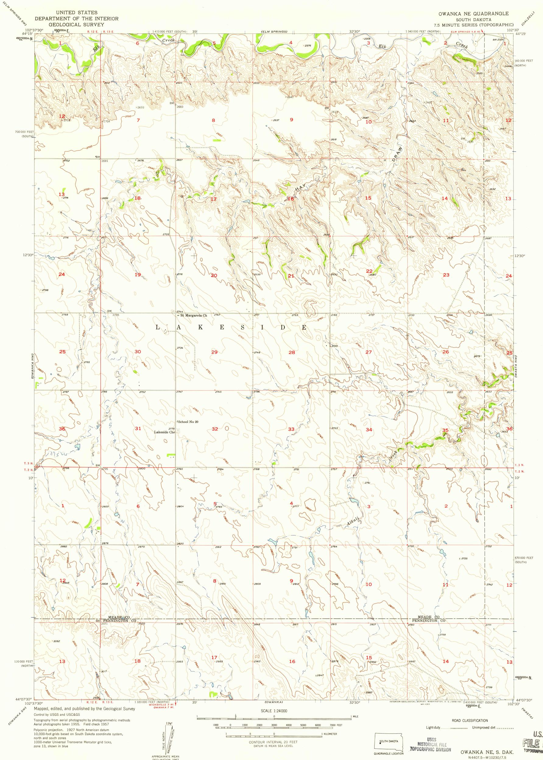
Polyconic projection. 1927 North American datum 10,000-foot grids based on South Dakota coordinate system, north and south zones 1000-meter Universal Transverse Mercator grid ticks, zone 13, shown in blue
