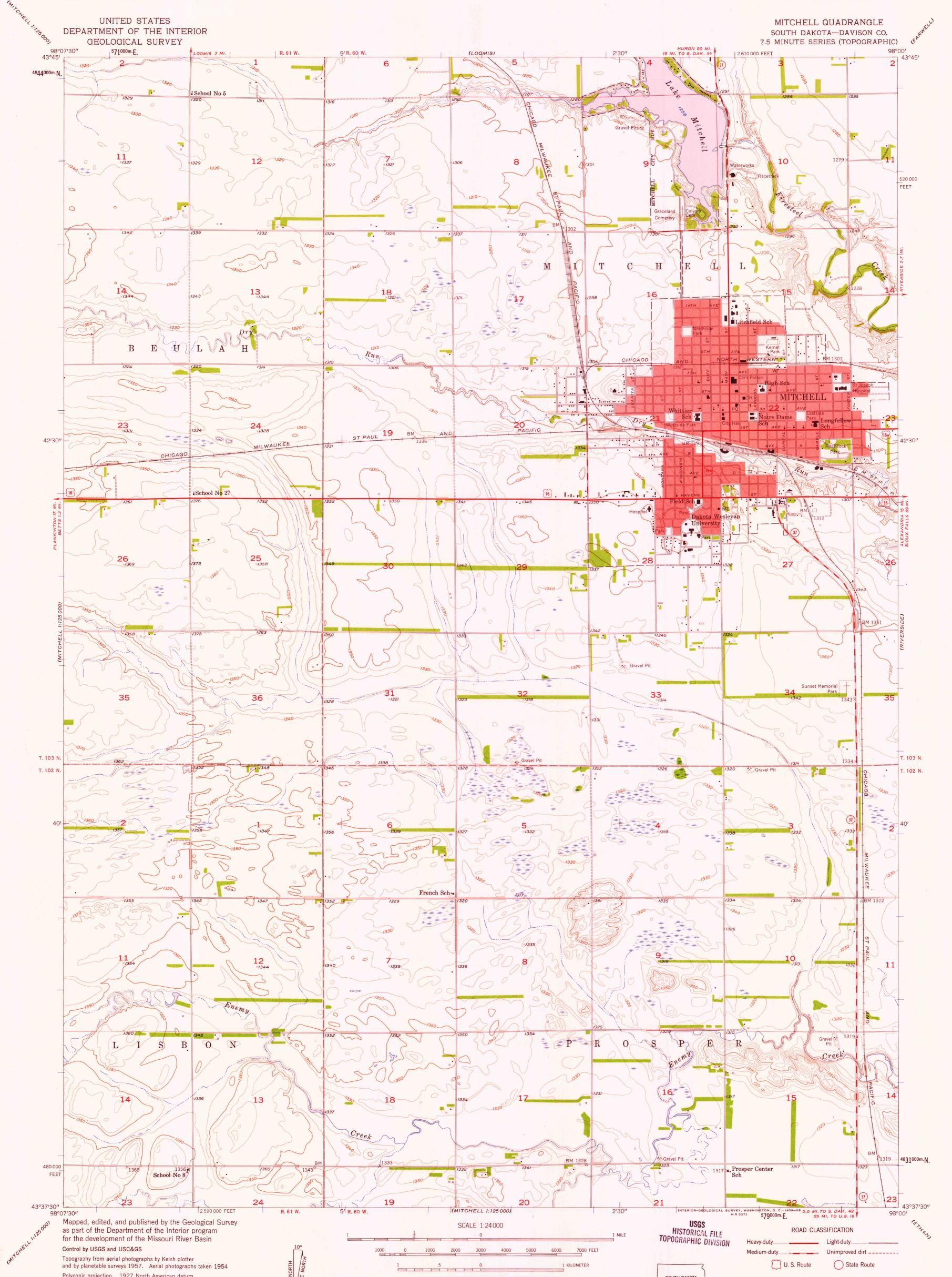
and by planetable surveys 1957. Aerial photographs taken 1954 Polyconic projection. 1927 North American datum 10,000-foot grid based on South Dakota coordinate system, south zone 1000-meter Universal Transverse Mercator grid ticks, zone 14, shown in blue Red tint indicates areas in which only landmark buildings are shown
