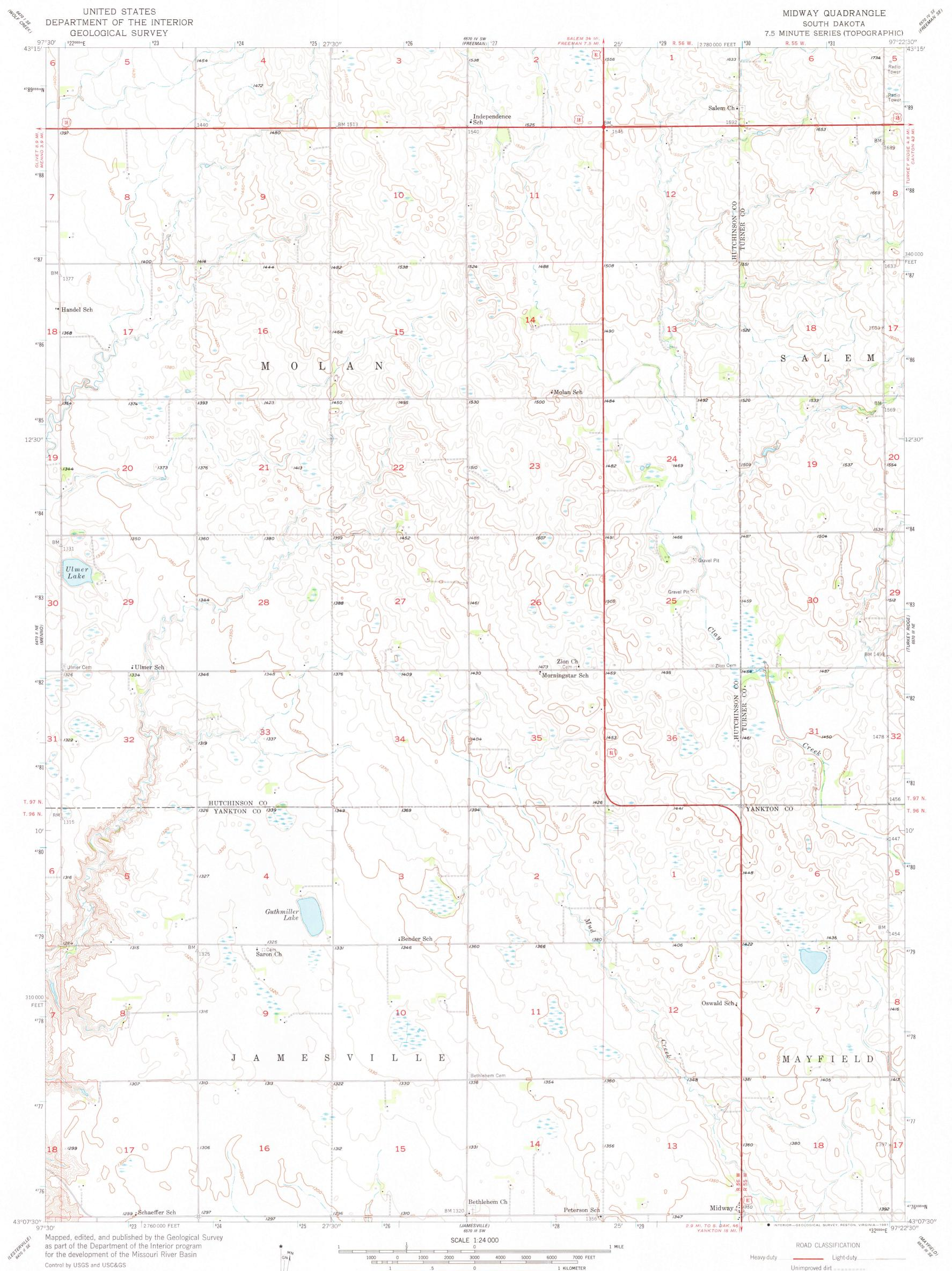
Topography from aerial photographs by Kelsh plotter Aerial photographs taken 1954. Field check 1957 Polyconic projection. 1927 North American datum 10,000-foot grid based on South Dakota coordinate system, south zone 1000-meter Universal Transverse Mercator grid ticks, zone 14, shown in blue To place on the predicted North American Datum 1983 move the projection lines 6 meters north and 28 meters east as shown by dashed corner ticks
