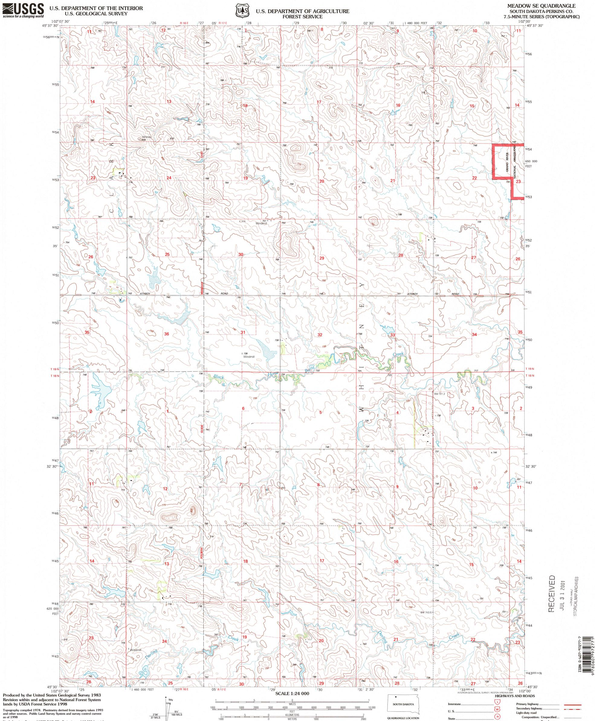
North American Datum of 1927 (NAD 27). Projection and 10 000-foot ticks: South Dakota coordinate system, north zone (Lambert conformal conic) Blue 1000-meter Universal Transverse Mercator ticks, zone 13
