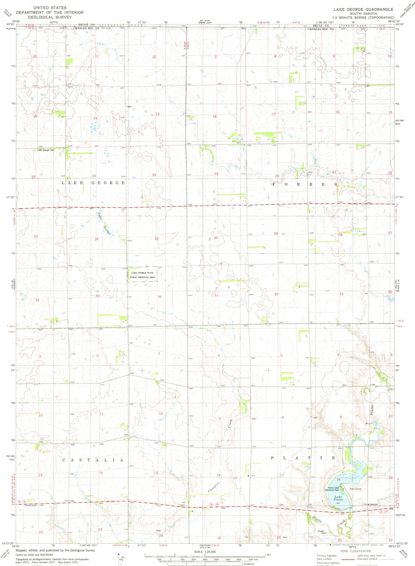
Projection and 10,000-foot grid ticks: South Dakota coordinate system, south zone (Lambert conformal conic) 1000-meter Universal Transverse Mercator grid, zone 14 1927 North American datum To place on the predicted North American Datum 1983 move the projection lines 6 meters north and 32 meters east as shown by dashed corner ticks
