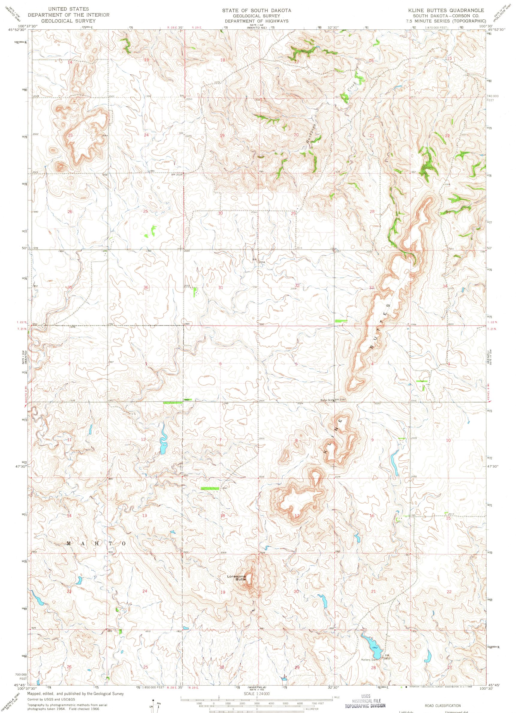
Polyconic projection. 1927 North American datum 10,000-foot grid based on South Dakota coordinate system, north zone 1000-meter Universal Transverse Mercator grid ticks, zone 14, shown in blue
