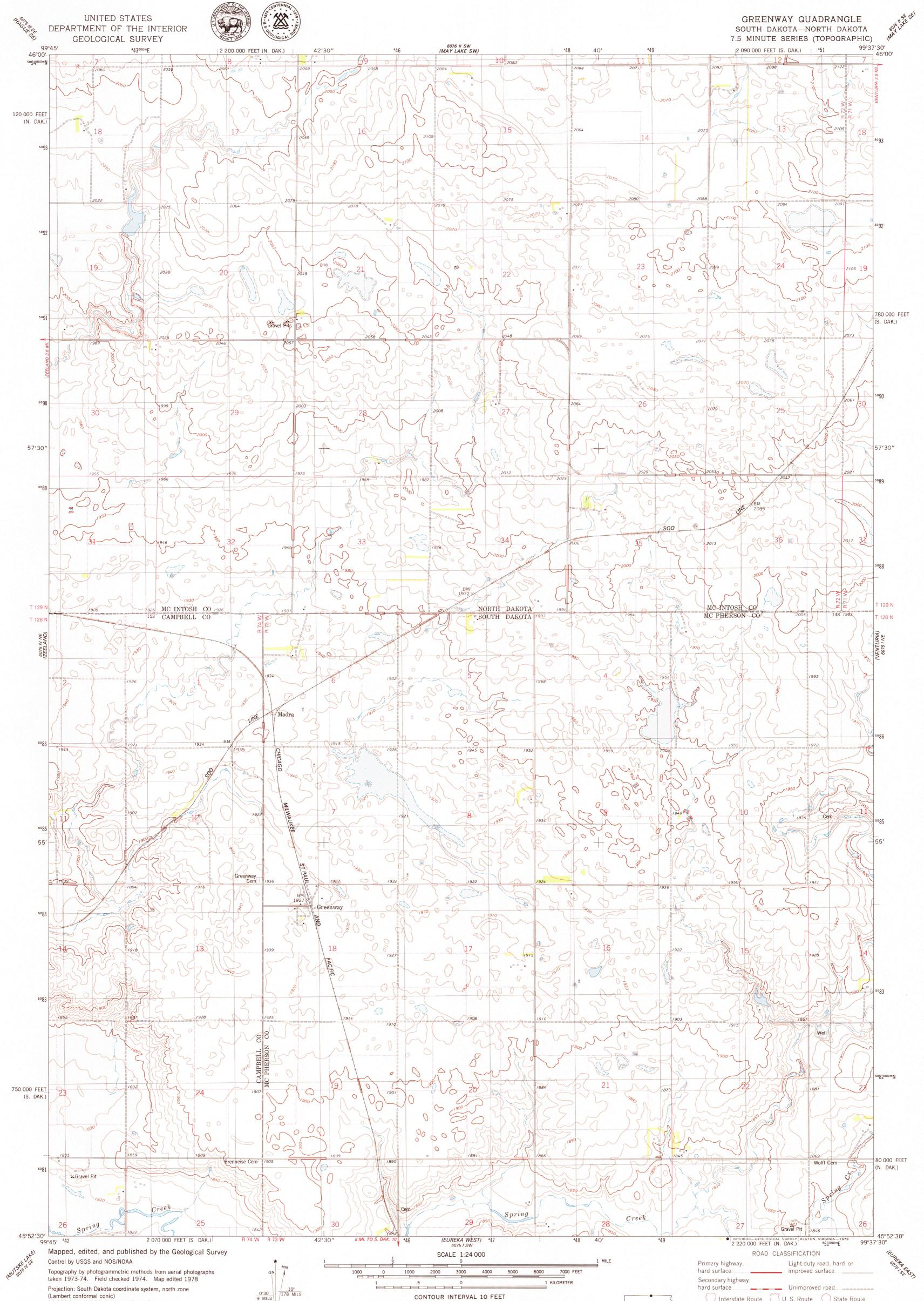
(Lambert conformal conic) 10,000-foot grid ticks based on South Dakota coordinate system, north zone and North Dakota coordinate system, south zone 1000-meter Universal Transverse Mercator grid, zone 14 UTM GRID AND 1978 MAGNETIC NORTH DECLINATION AT CENTER OF SHEET 1927 North American datum Fine red dashed lines indicate selected fence and field lines where generally visible on aerial photographs. This information is unchecked
