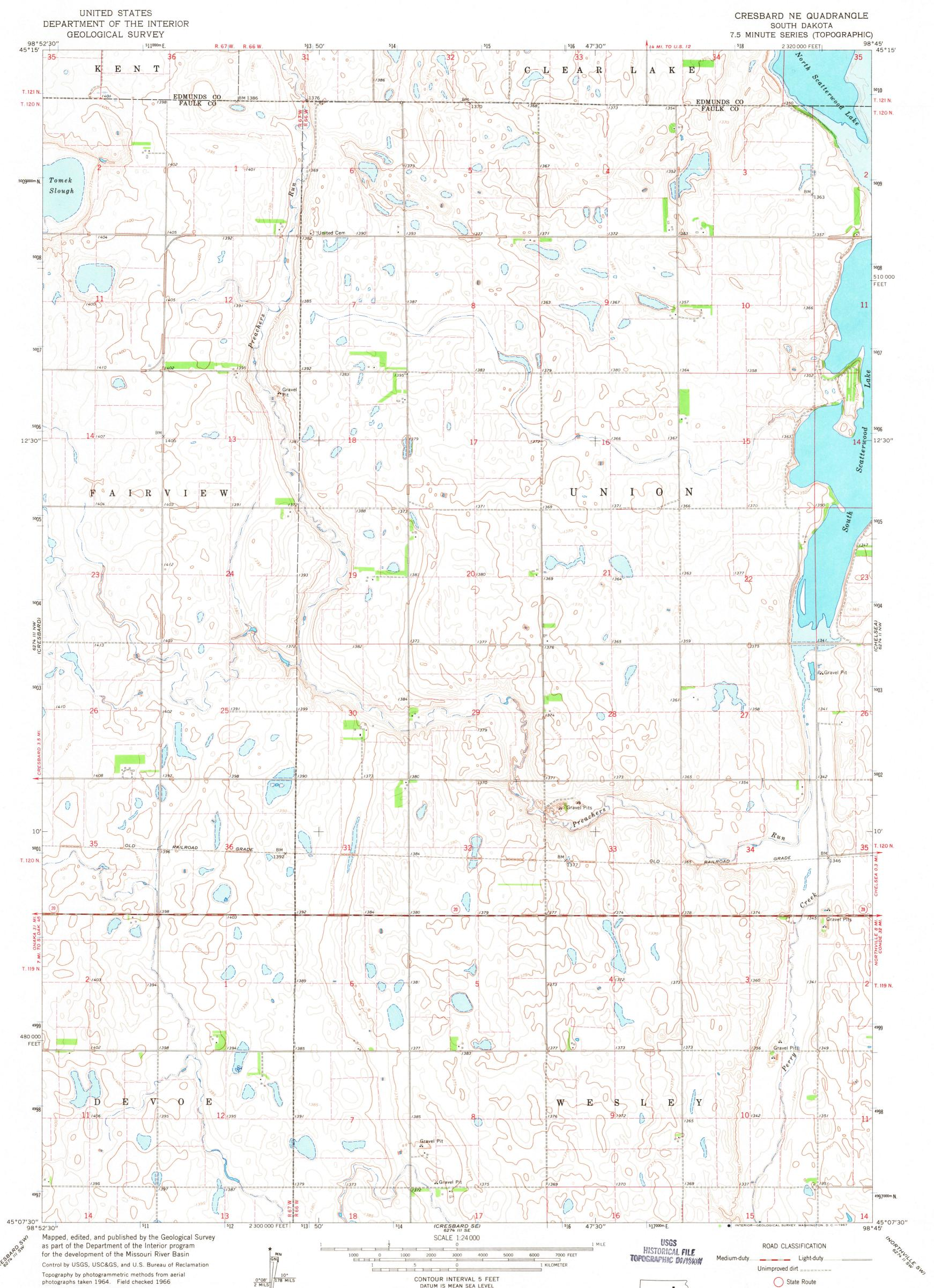
Polyconic projection. 1927 North American datum 10,000-foot grid based on South Dakota coordinate system, north zone 1000-meter Universal Transverse Mercator grid ticks, UTM GRID AND 1966 MAGNETIC NORTH DECLINATION AT CENTER OF SHEET zone 14, shown in blue
