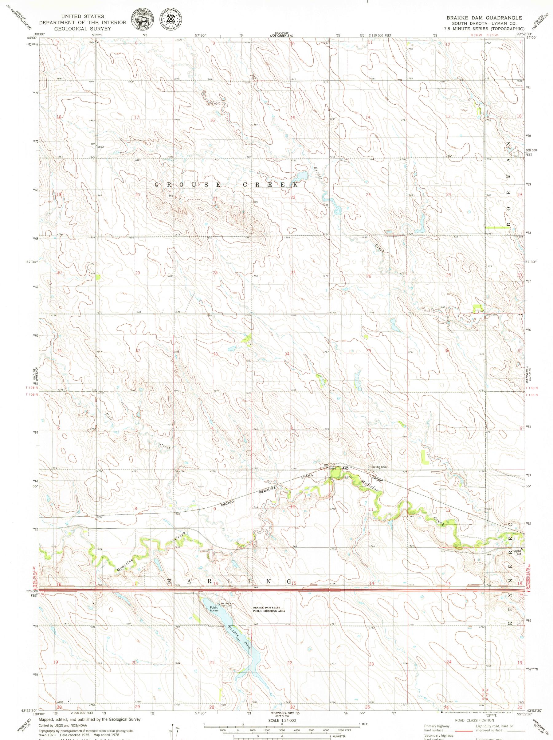
Projection and 10,000-foot grid ticks: South Dakota coordinate system, south zone (Lambert conformal conic) 1000-meter Universal Transverse Mercator grid, zone 14 1927 North American datum
