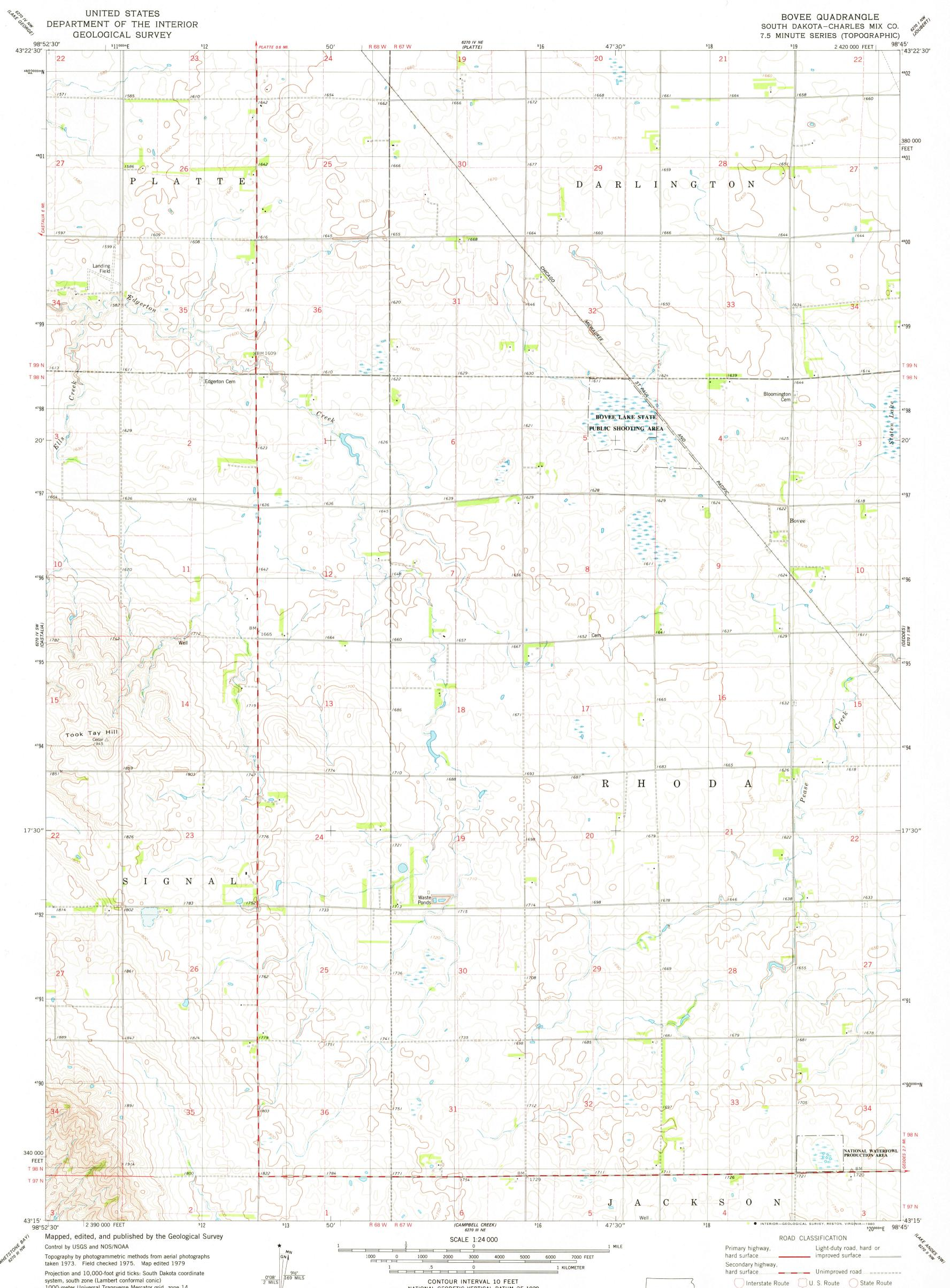
Projection and 10,000-foot grid ticks: South Dakota coordinate system, south zone (Lambert conformal conic) 1000-meter Universal Transverse Mercator grid, zone 14 1927 North American datum To place on the predicted North American Datum 1983 move the projection lines 6 meters north and 31 meters east as shown by dashed corner ticks
