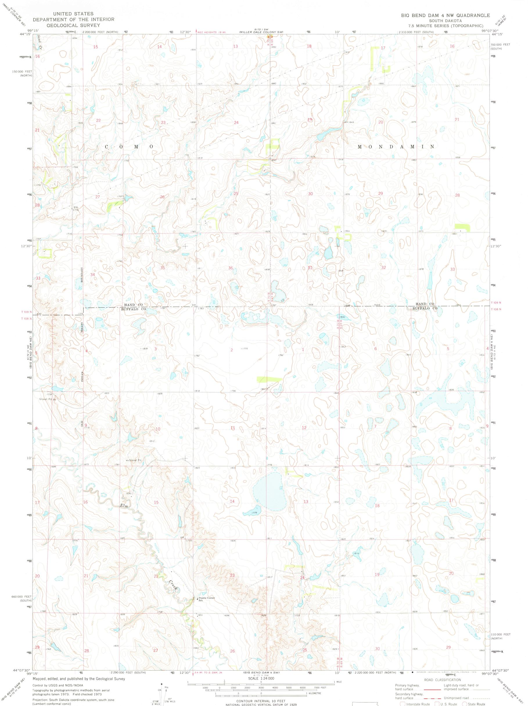
Projection: South Dakota coordinate system, south zone (Lambert conformal conic) 10,000-foot grid ticks based on South Dakota coordinate system, south and north zones 1000-metre Universal Transverse Mercator grid ticks, zone 14, shown in blue. 1927 North American datum
