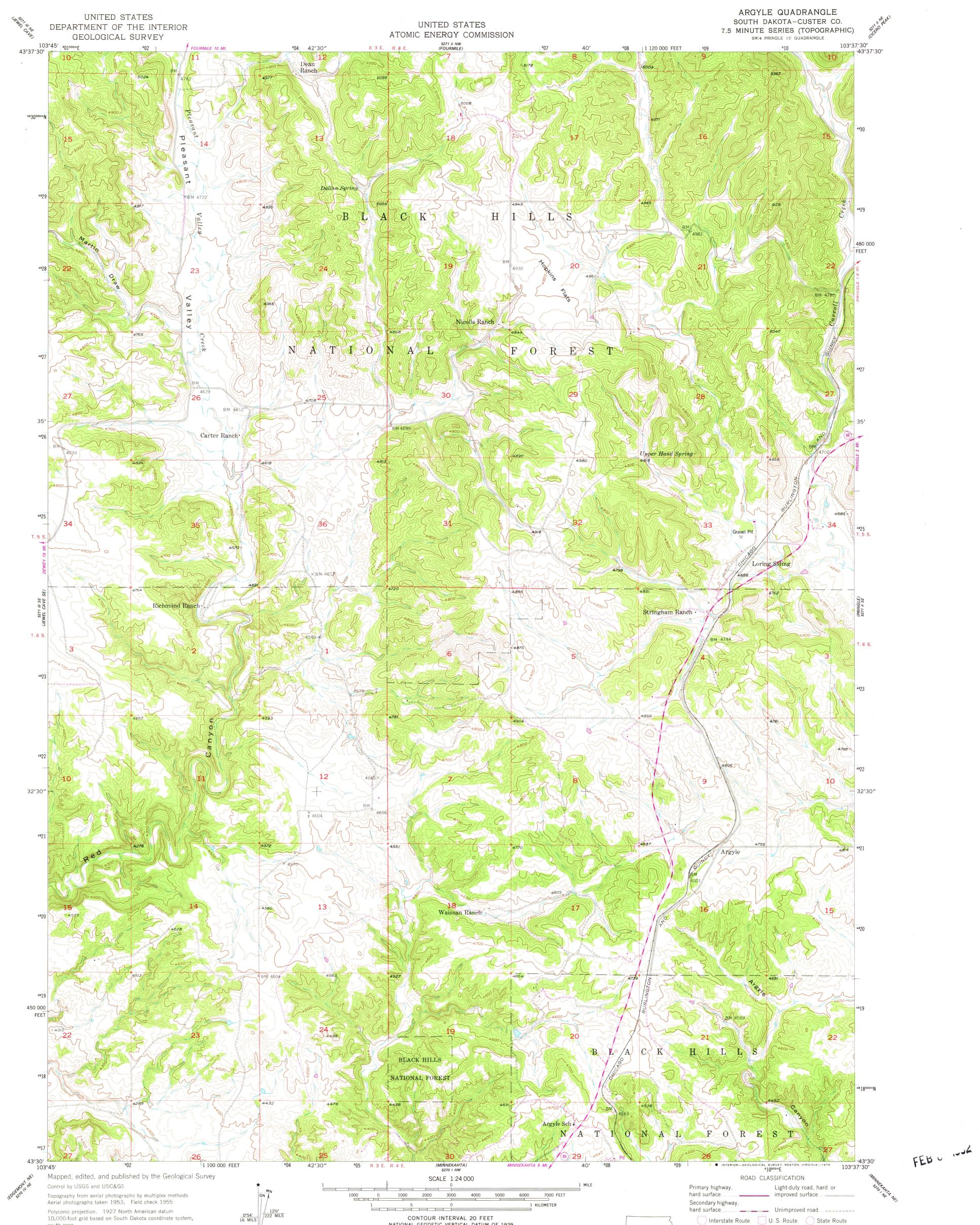
Polyconic projection. 1927 North American datum 10,000-foot grid based on South Dakota coordinate system, south zone To place on the predicted North American Datum 1983 move the projection lines 6 meters north and 43 meters east as shown by dashed corner ticks 1000-meter Universal Transverse Mercator grid ticks, zone 13, shown in blue
