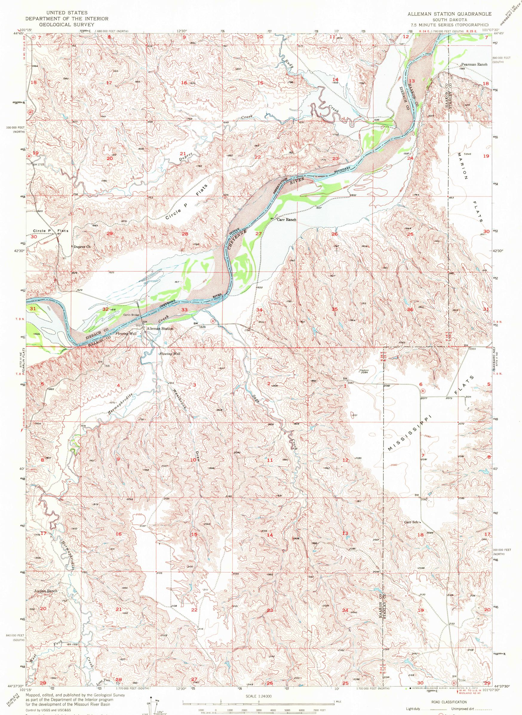
Control by USGS and USC&GS Topography from aerial photographs by multiplex methods and by planetable surveys 1956. Aerial photographs taken 1948 Polyconic projection. 1927 North American datum 10,000-foot grids based on South Dakota coordinate system, north and south zones 1000-meter Universal Transverse Mercator grid ticks, zone 14, shown in blue Areas covered by dashed light-blue pattern to be submerged by Oahe Reservoir Elevation flood control pool 1620
