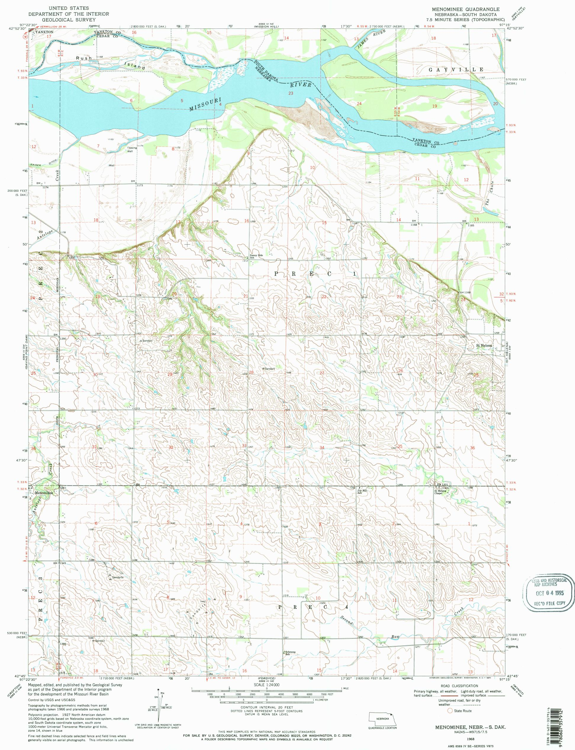
photographs taken 1966 and planetable surveys 1968 Polyconic projection. 1927 North American datum 10,000-foot grids based on Nebraska coordinate system, north zone and South Dakota coordinate system, south zone UTM GRID AND 1968 MAGNETIC NORTH DECLINATION AT CENTER OF SHEET 1000-meter Universal Transverse Mercator grid ticks, zone 14, shown in blue
