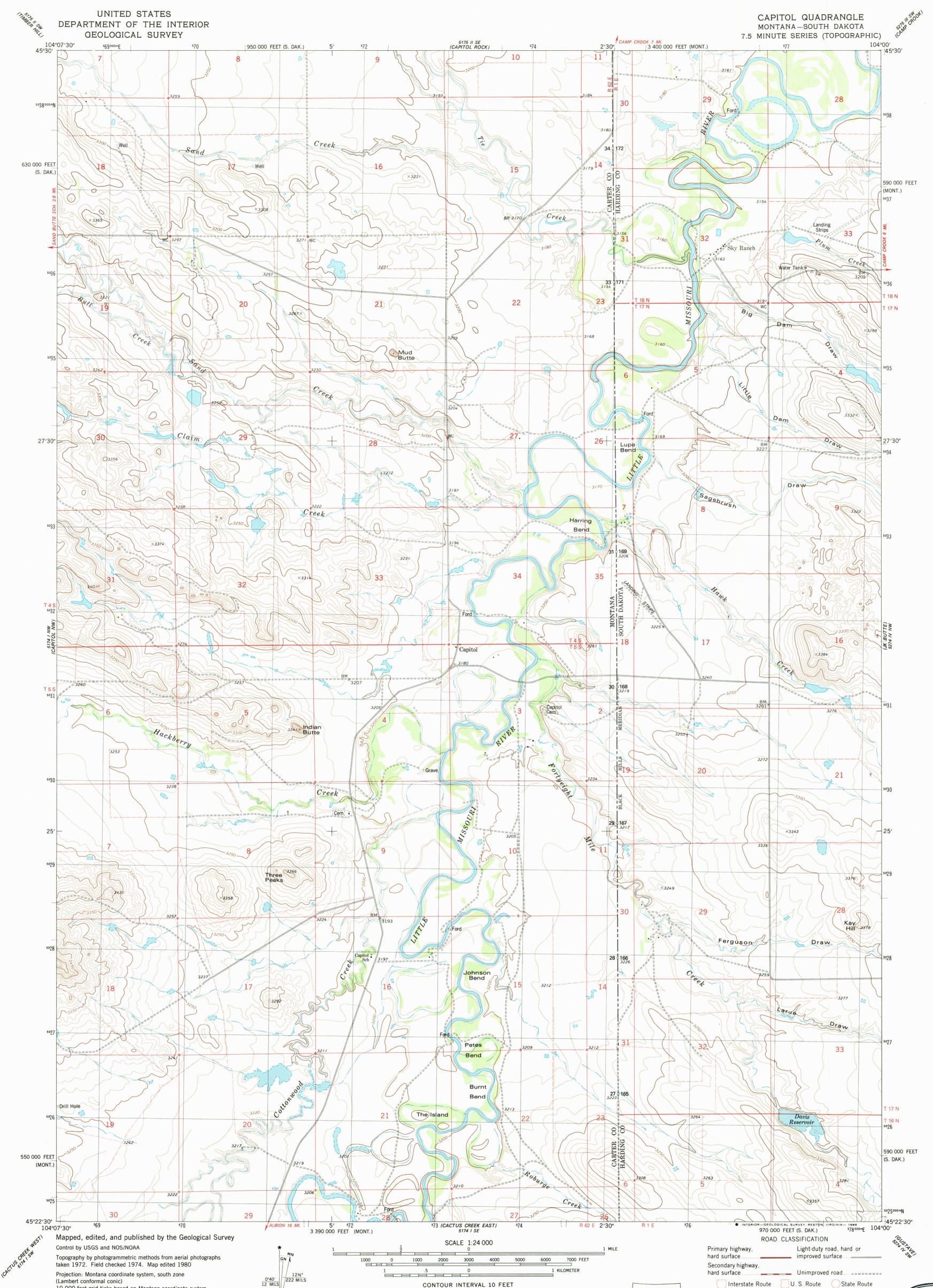
(Lambert conformal conic) 10,000-foot grid ticks based on Montana coordinate system, south zone and South Dakota coordinate system, north zone 1000-meter Universal Transverse Mercator grid, zone 13 1927 North American Datum To place on the predicted North American Datum 1983 move the projection lines 4 meters north and 40 meters east as shown by dashed corner ticks
