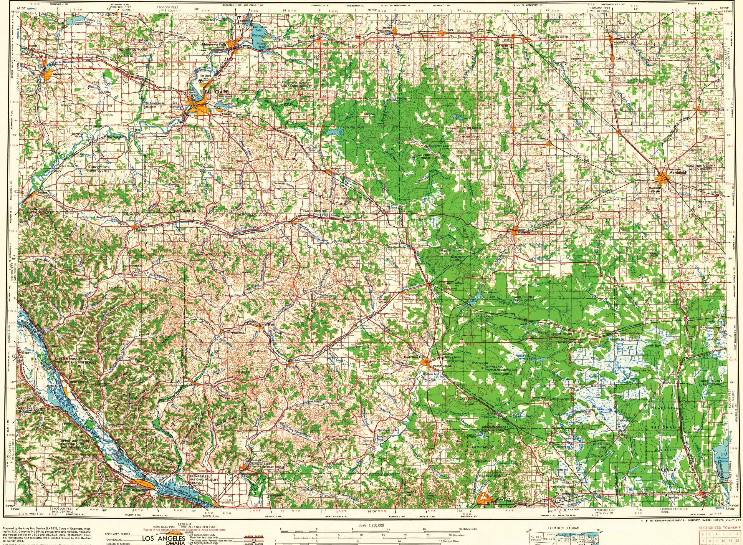
100,000-foot grids based on Wisconsin coordinate system, central and south zones and Minnesota coordinate system, south zone.  $10,000\,\mathrm{meter}$  Universal Transverse Mercator grid ticks, zone 15, shown in blue.
