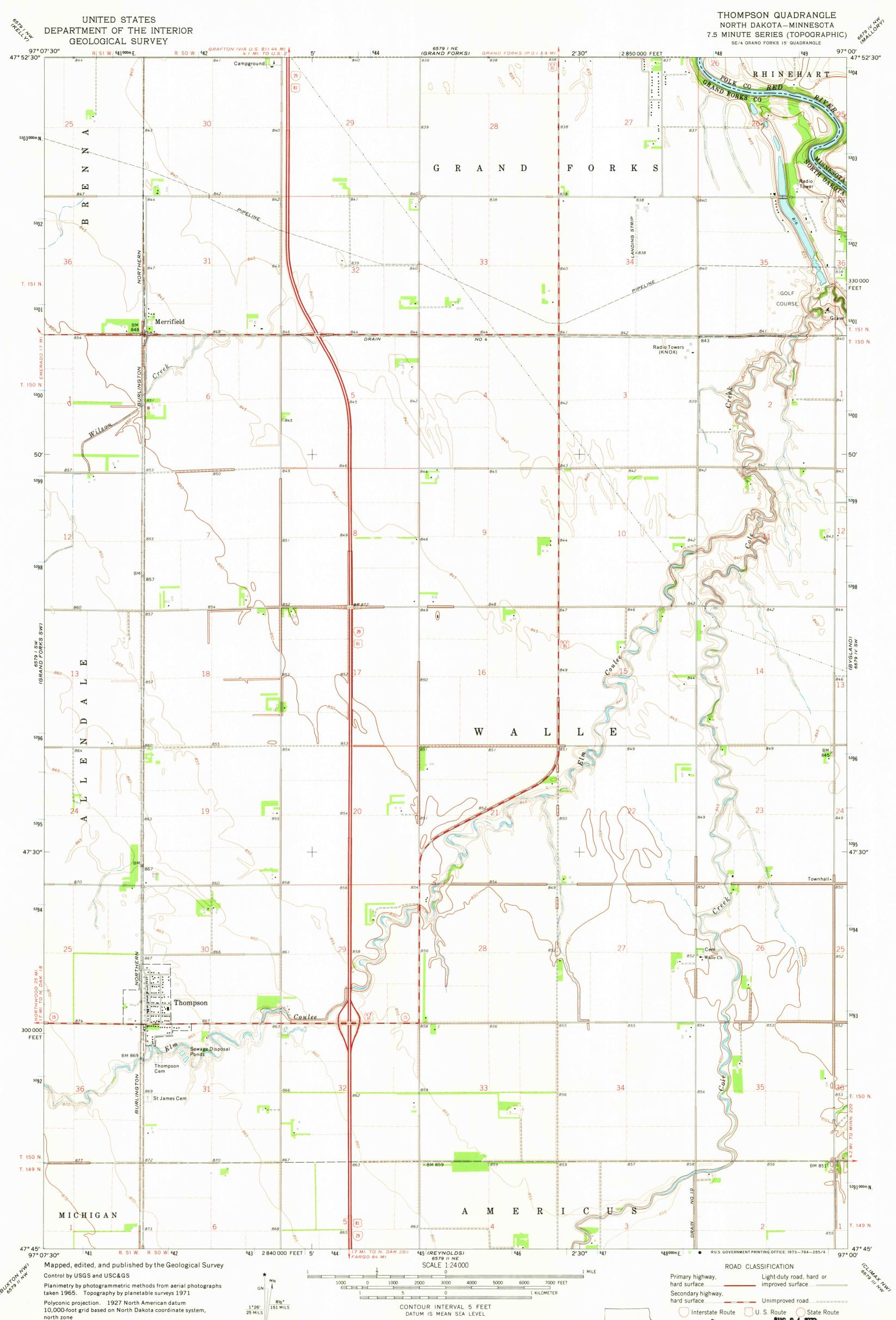
Polyconic projection. 1927 North American datum 10,000-foot grid based on North Dakota coordinate system, north zone 1000-meter Universal Transverse Mercator grid ticks, zone 14, shown in blue Fine red dashed lines indicate selected fence and field lines
