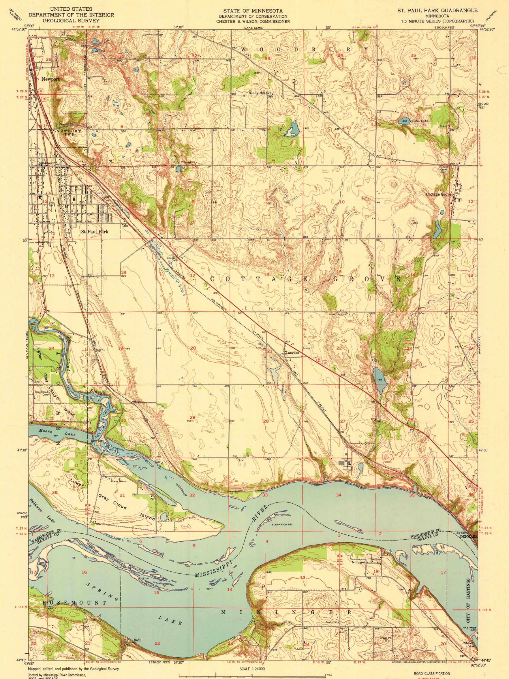
USGS, and USC&GS Topography from aerial photographs by multiplex methods Aerial photographs taken 1947. Field check 1950 Polyconic projection. 1927 North American datum 10,000-foot grid based on Minnesota coordinate system, south zone
