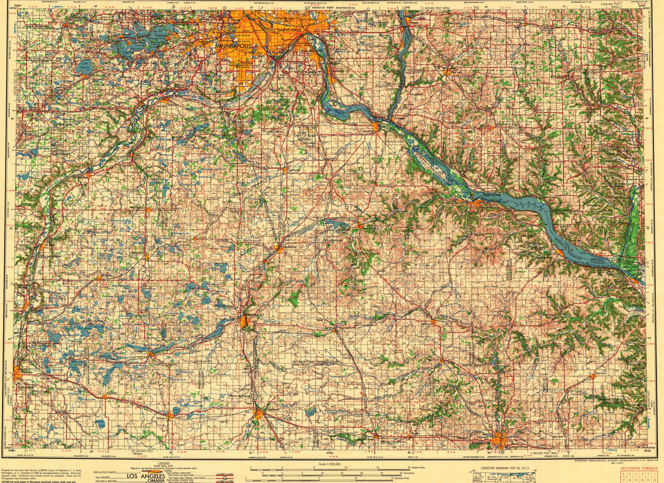
Prepared by the Army Map Service (LKBPM), Corps of Engineers, U. S. Army, Washington, D. C. Compiled in 1956 by photogrammetric methods. Aerial photography 1953. Horizontal and vertical control by USC&GS, USGS and CE. 100,000-foot grids based on Minnesota coordinate system, south zone and
