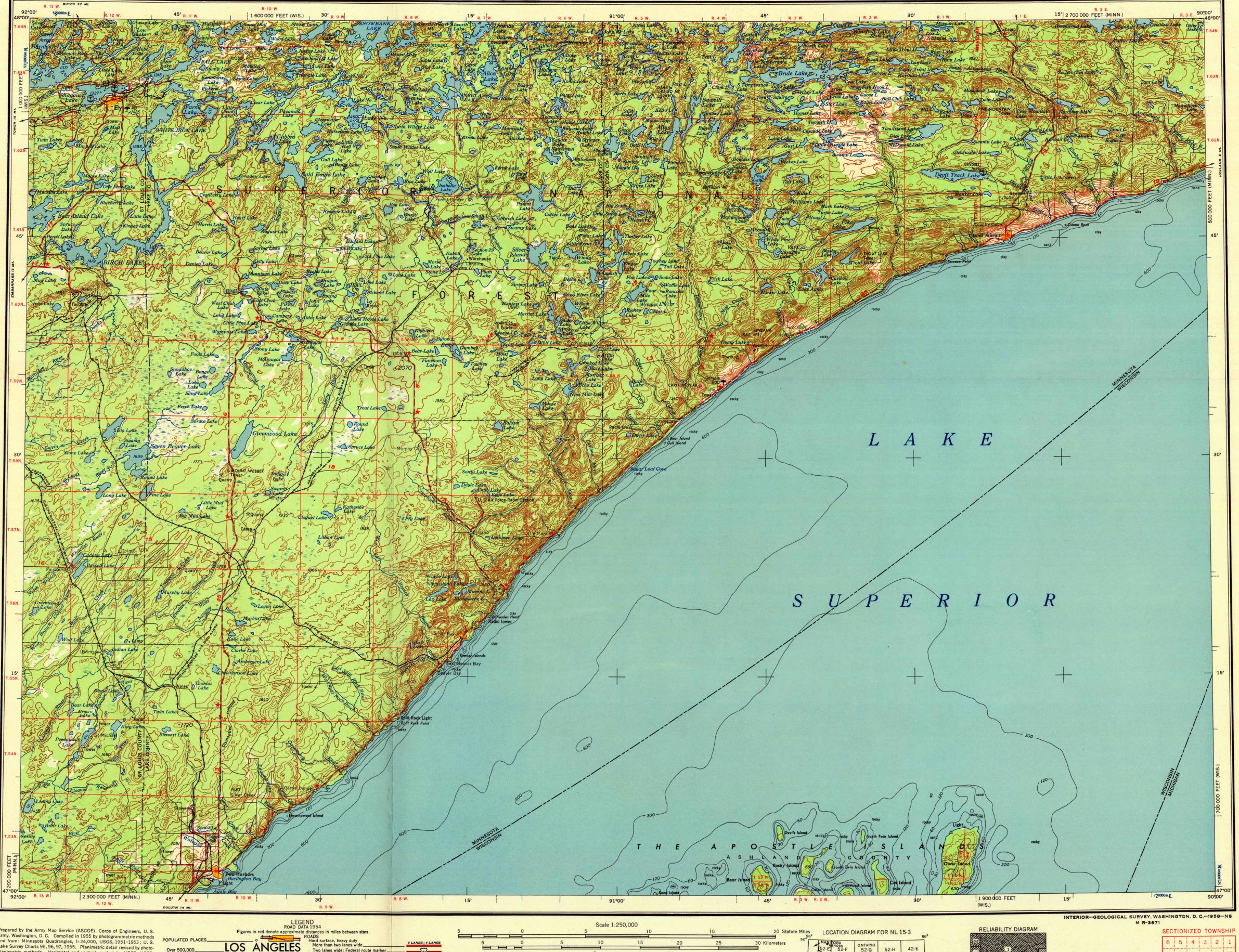
Prepared by the Army Map Service (ASCGE), Corps of Engineers, U. S. Army, Washington, D. C. Compiled in 1955 by photogrammetric methods and from: Minnesota Quadrangles, 1:24,000, USGS, 1951–1953; U. S. Lake Survey Charts 95, 96, 97, 1955. Planimetric detail revised by photoplanimetric methods. Horizontal and vertical control by USGS, USFS, and USC&GS. Photography field annotated 1954.
