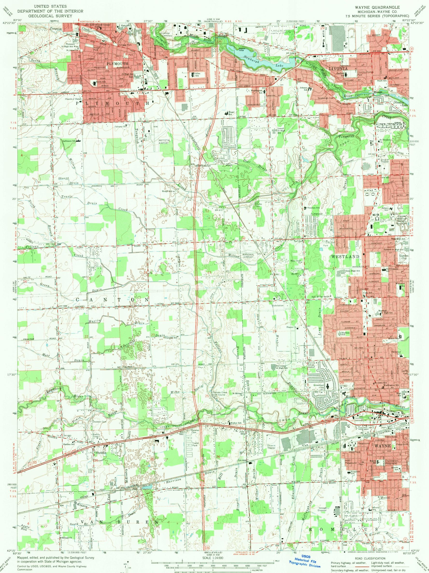
Planimetry by photogrammetric methods from aerial photographs Topography by planetable surveys 1940–41. Revised from aerial photographs taken 1966–67. Field checked 1968
