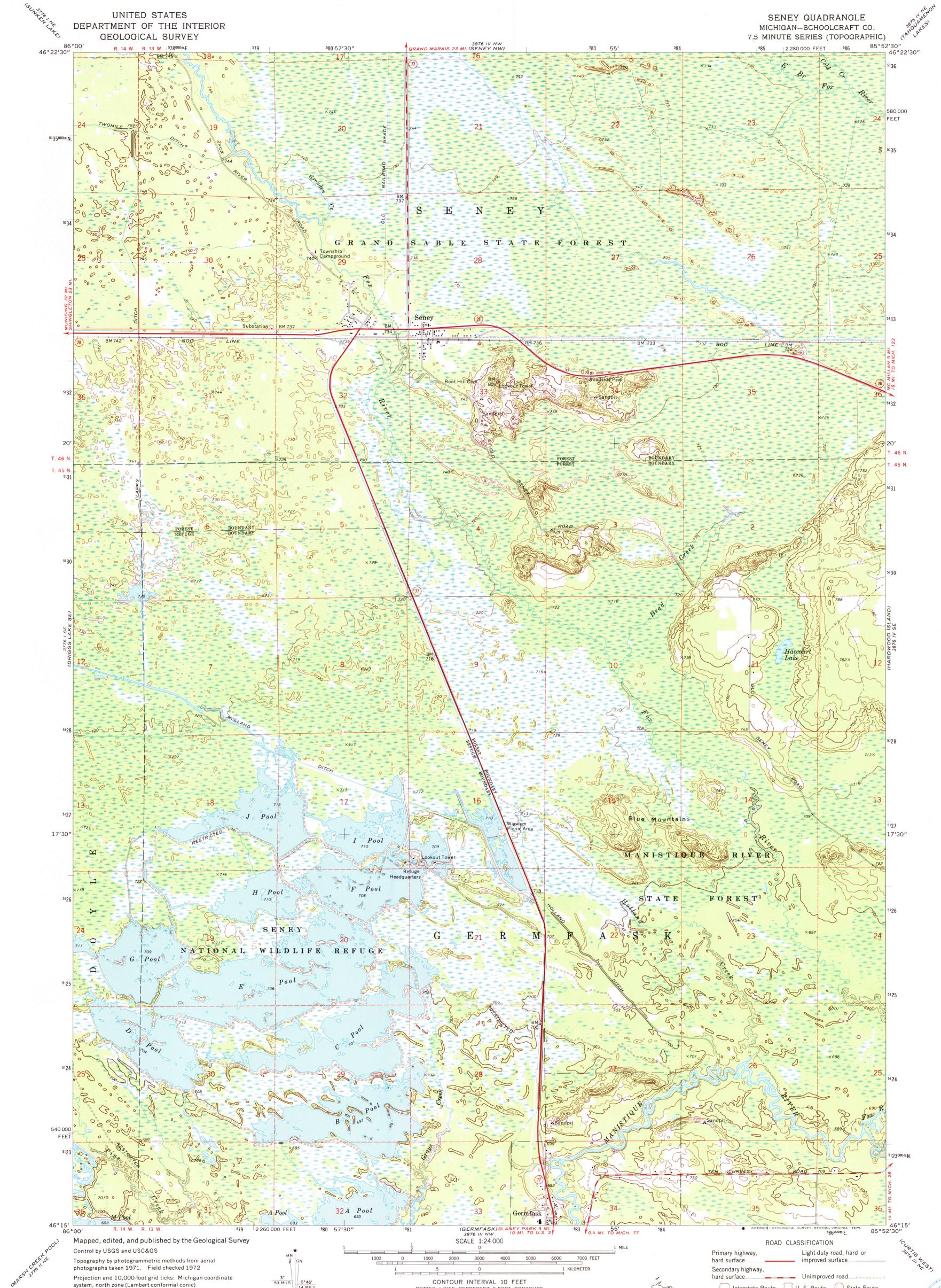
Projection and 10,000-foot grid ticks: Michigan coordinate system, north zone (Lambert conformal conic) 1000-meter Universal Transverse Mercator grid ticks, zone 16, shown in blue. 1927 North American datum
