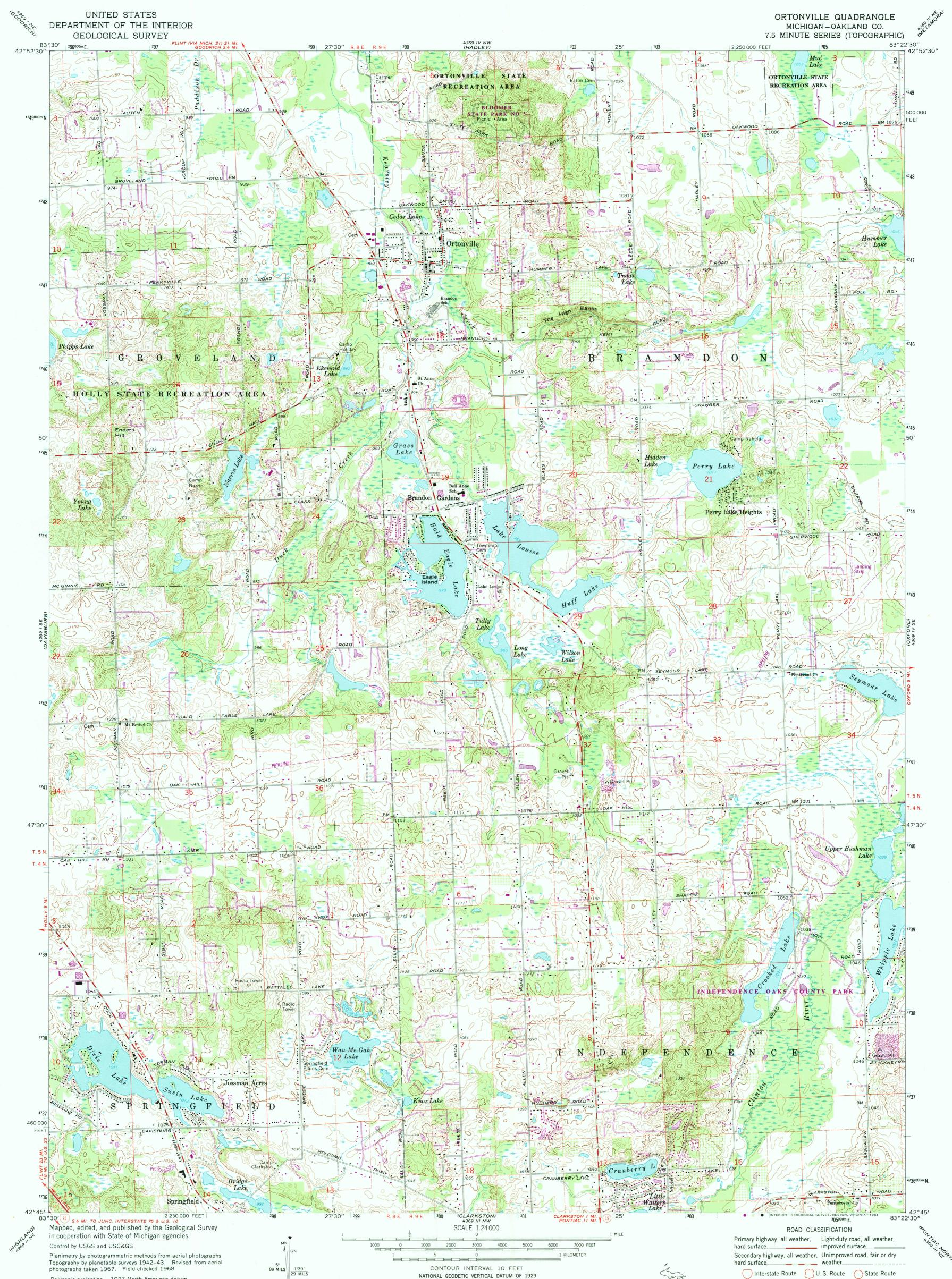
Polyconic projection. 1927 North American datum 10,000-foot grid based on Michigan coordinate system, south zone 1000-meter Universal Transverse Mercator grid ticks, zone 17, shown in blue To place on the predicted North American Datum 1983, move the projection lines 6 meters west as shown by dashed corner ticks
