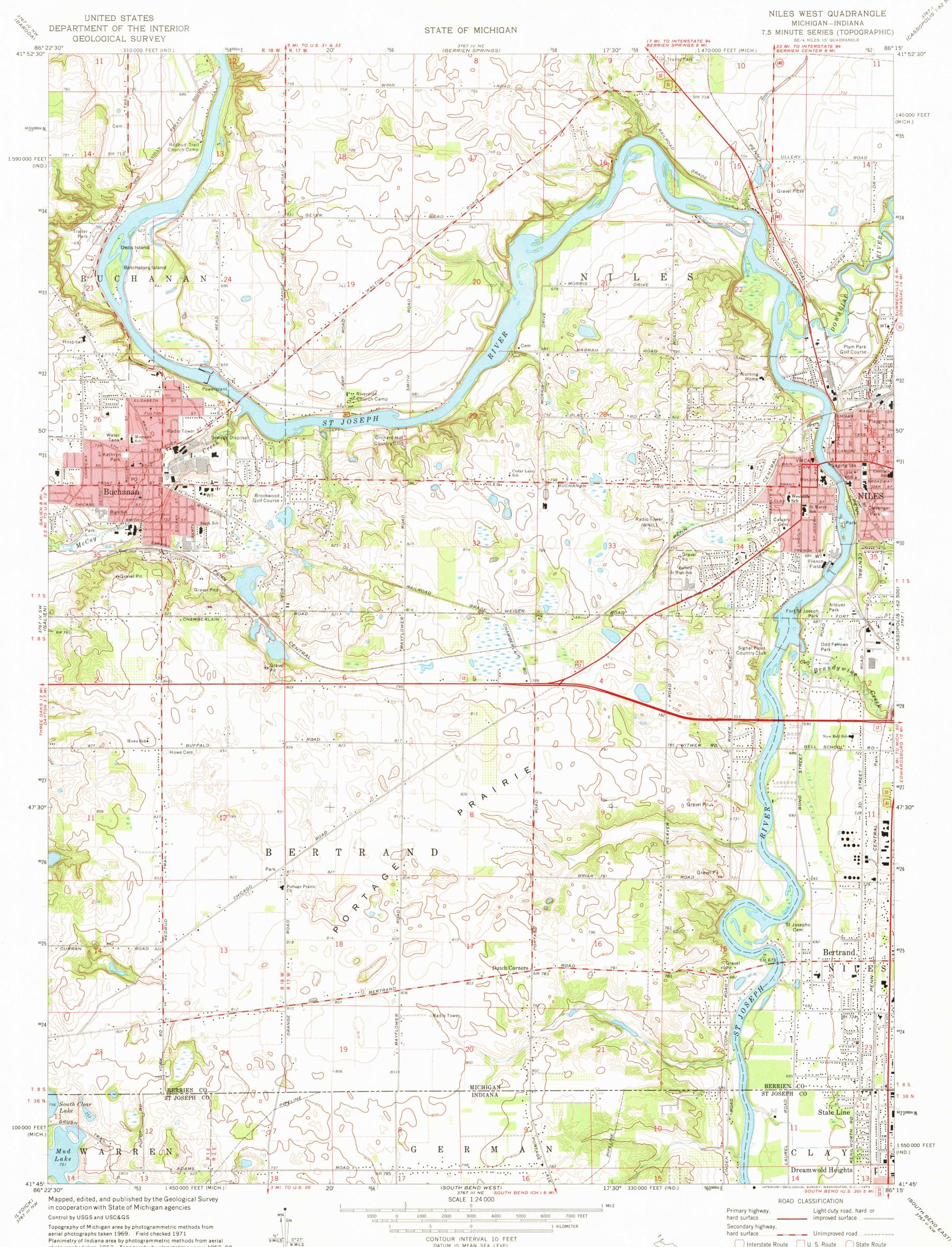
Planimetry of Indiana area by photogrammetric methods from aerial photographs taken 1952. Topography by planetable surveys 1957-58 Revised from aerial photographs taken 1969. Field checked 1971
