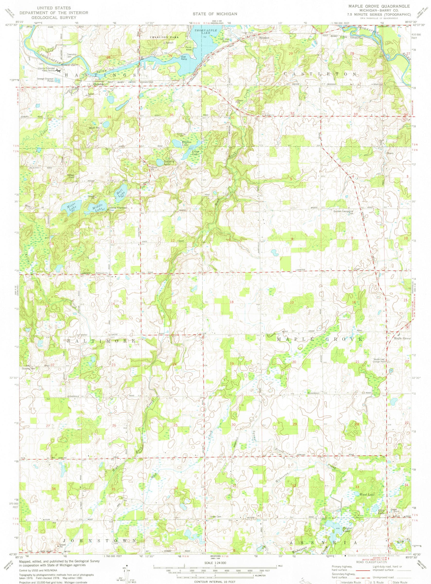
Projection and 10,000-foot grid ticks: Michigan coordinate system, south zone (Lambert conformal conic) 1000-meter Universal Transverse Mercator grid, zone 16 1927 North American Datum To place on the predicted North American Datum 1983 move the projection lines 1 meter north as shown by dashed corner ticks
