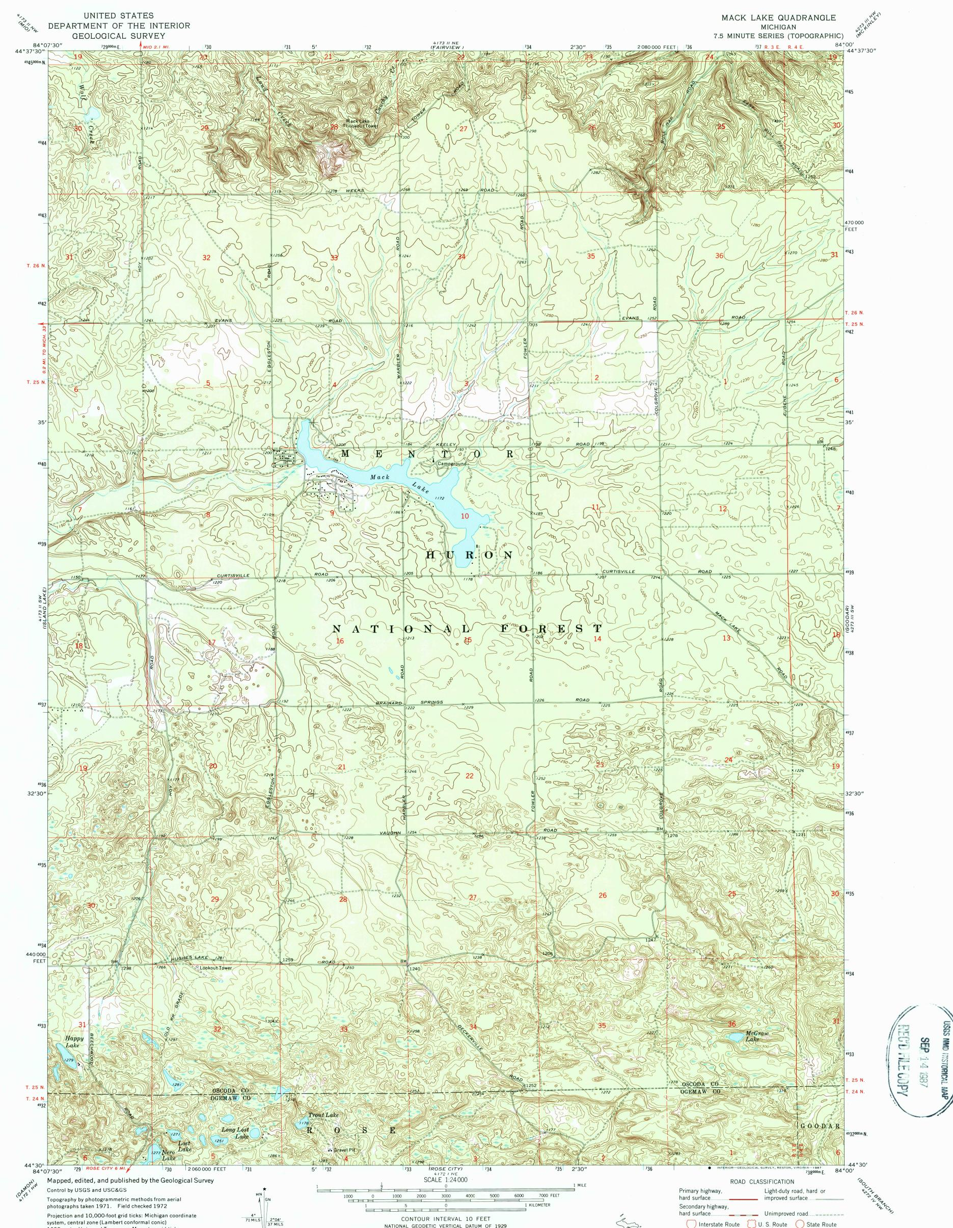
Projection and 10,000-foot grid ticks: Michigan coordinate system, central zone (Lambert conformal conic) 1000-meter Universal Transverse Mercator grid ticks, zone 16, shown in blue. 1927 North American datum
