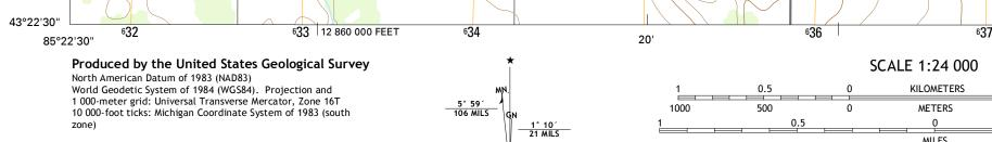
UTM GRID AND 2014 MAGNETIC NORTH DECLINATION AT CENTER OF SHEET
