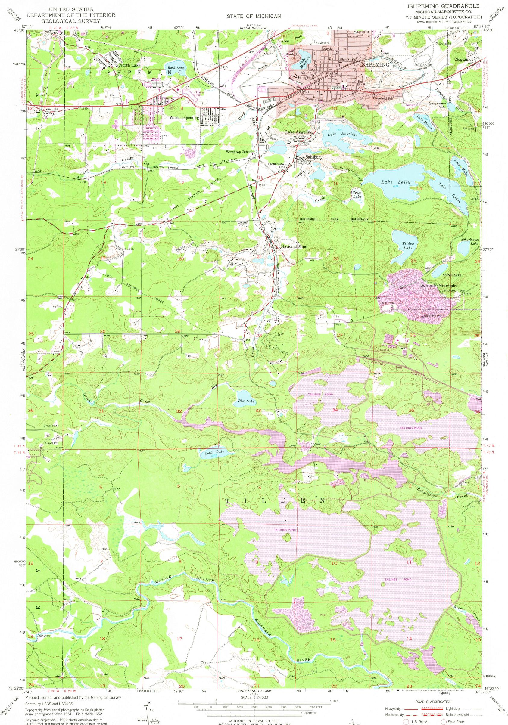
Polyconic projection. 1927 North American datum 10,000-foot grid based on Michigan coordinate system, north zone Red tint indicates area in which only landmark buildings are shown UTM GRID AND 1975 MAGNETIC NORTH DECLINATION AT CENTER OF SHEET 1000-metre Universal Transverse Mercator grid ticks, zone 16, shown in blue
