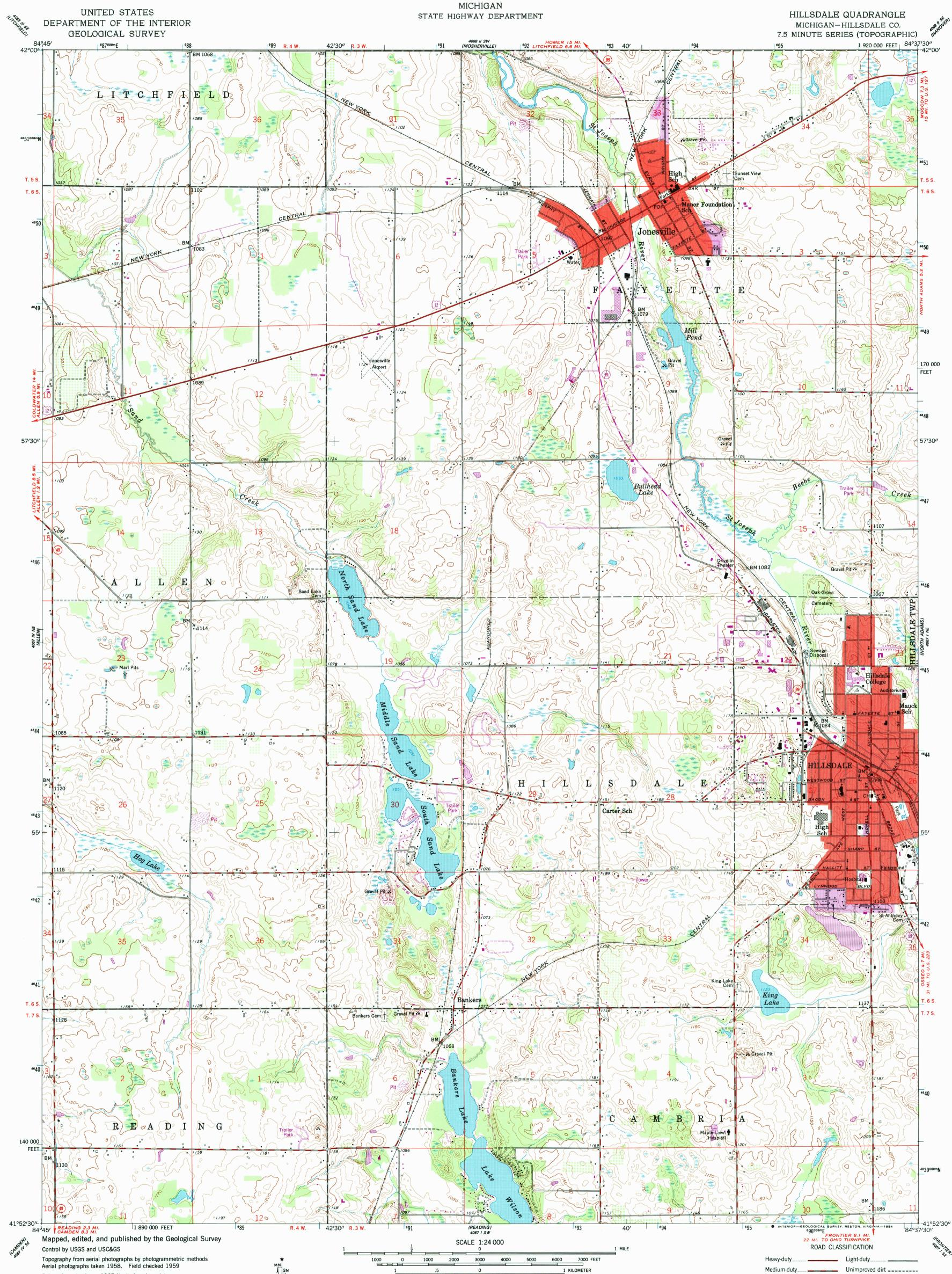
Polyconic projection. 1927 North American datum 10,000-foot grid based on Michigan coordinate system, south zone To place on the predicted North American Datum 1983 move the projection lines 0 meters north and 3 meters west as shown by dashed corner ticks 1000-meter Universal Transverse Mercator grid ticks, zone 16, shown in blue
