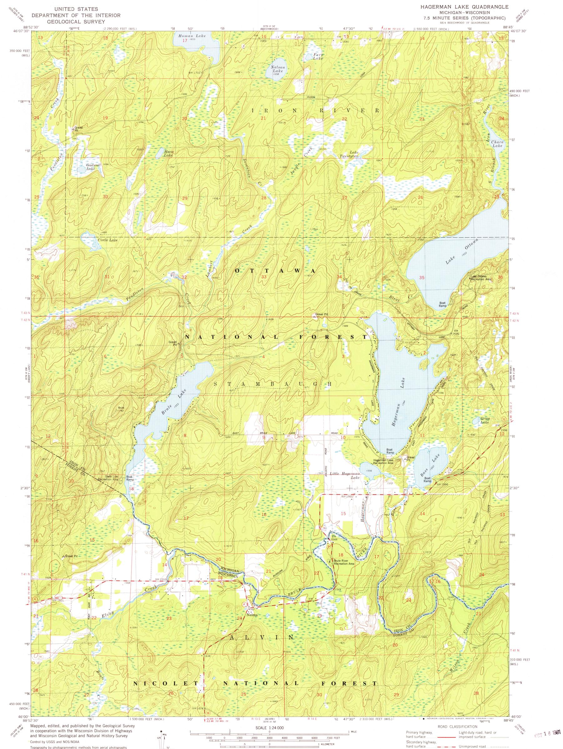
Topography by photogrammetric methods from aerial photographs taken 1976. Field checked 1978. Map edited 1981 Projection: Michigan coordinate system, north zone (Lambert conformal conic)
