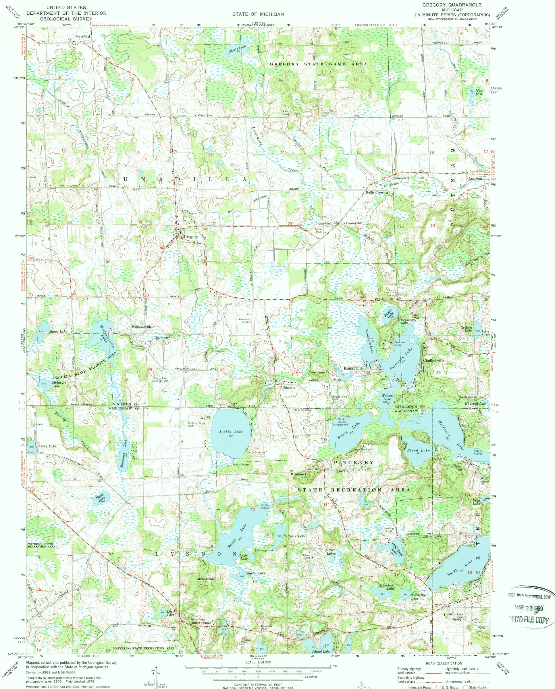
Projection and 10,000-foot grid ticks: Michigan coordinate system, south zone (Lambert conformal conic) 1000-metre Universal Transverse Mercator grid ticks, zone 16, shown in blue. 1927 North American datum
