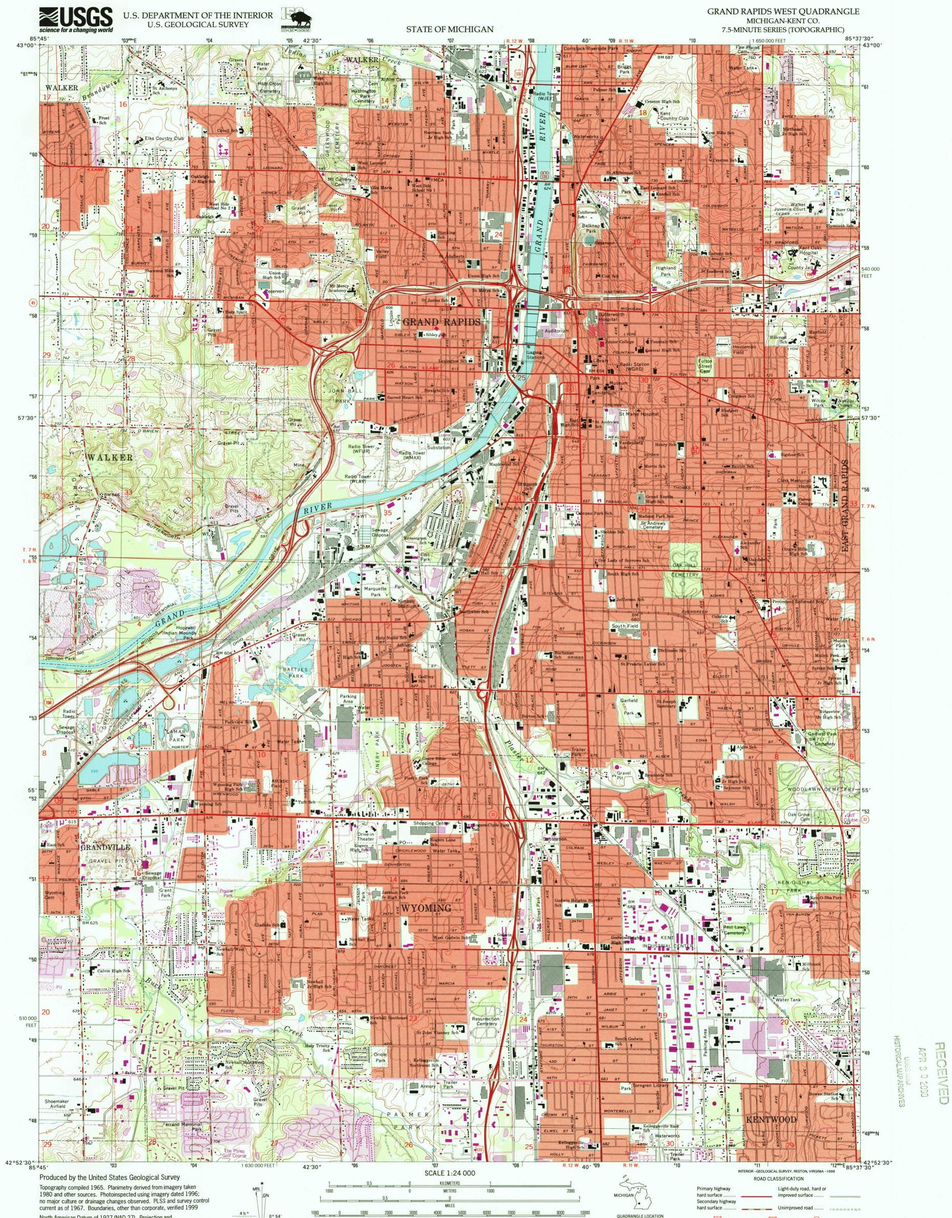
10 000-foot ticks: Michigan coordinate system, south zone (Lambert conformal conic) 1000-meter Universal Transverse Mercator grid, zone 16 North American Datum of 1983 (NAD 83) is shown by dashed corner ticks. The values of the shift between NAD 27 and NAD 83 for 7.5-minute intersections are obtainable from National Geodetic Survey NADCON software
