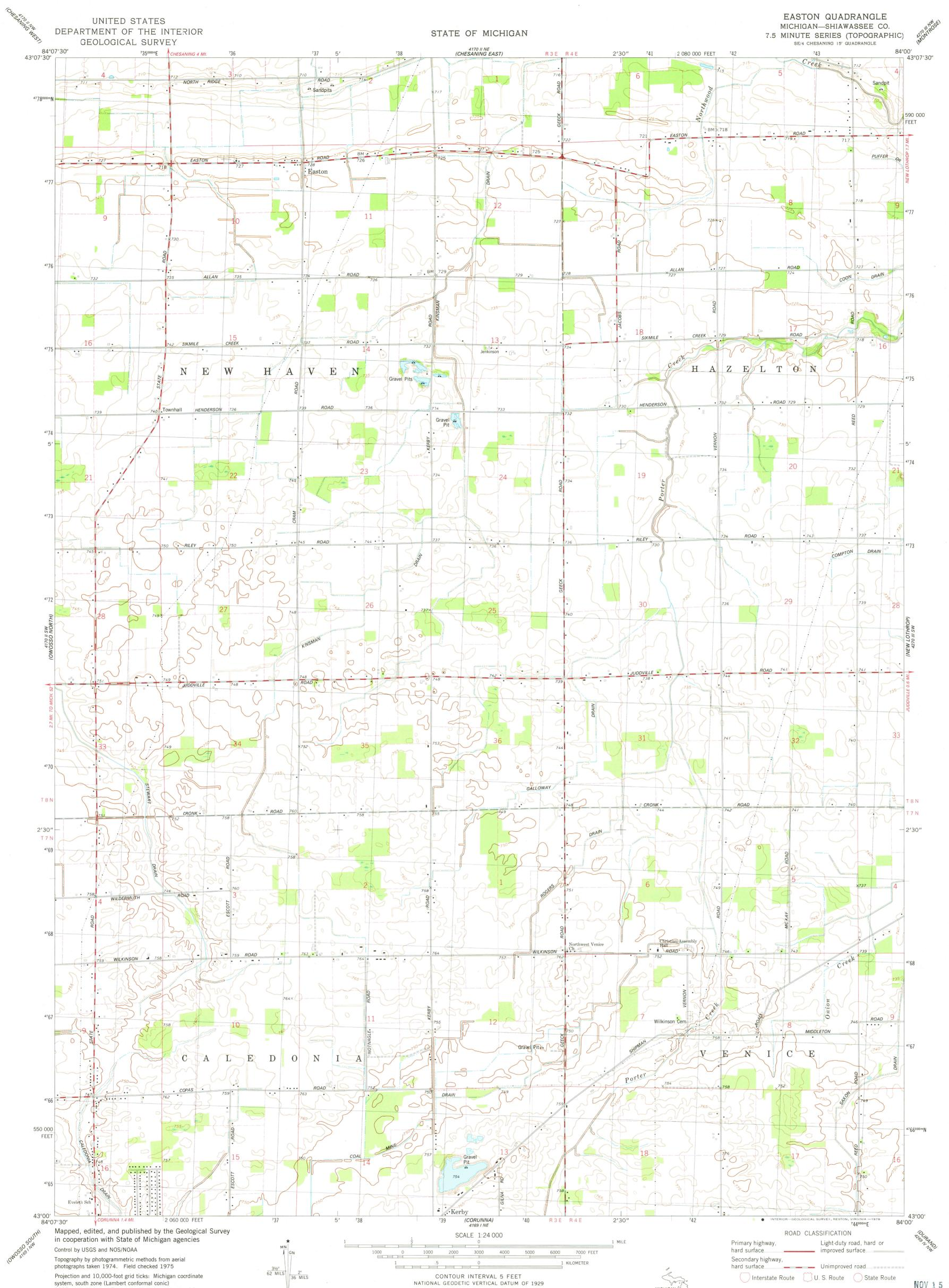
Projection and 10,000-foot grid ticks: Michigan cocrdinate system, south zone (Lambert conformal conic) 1000-meter Universal Transverse Mercator grid, zone 16 1927 North American datum
