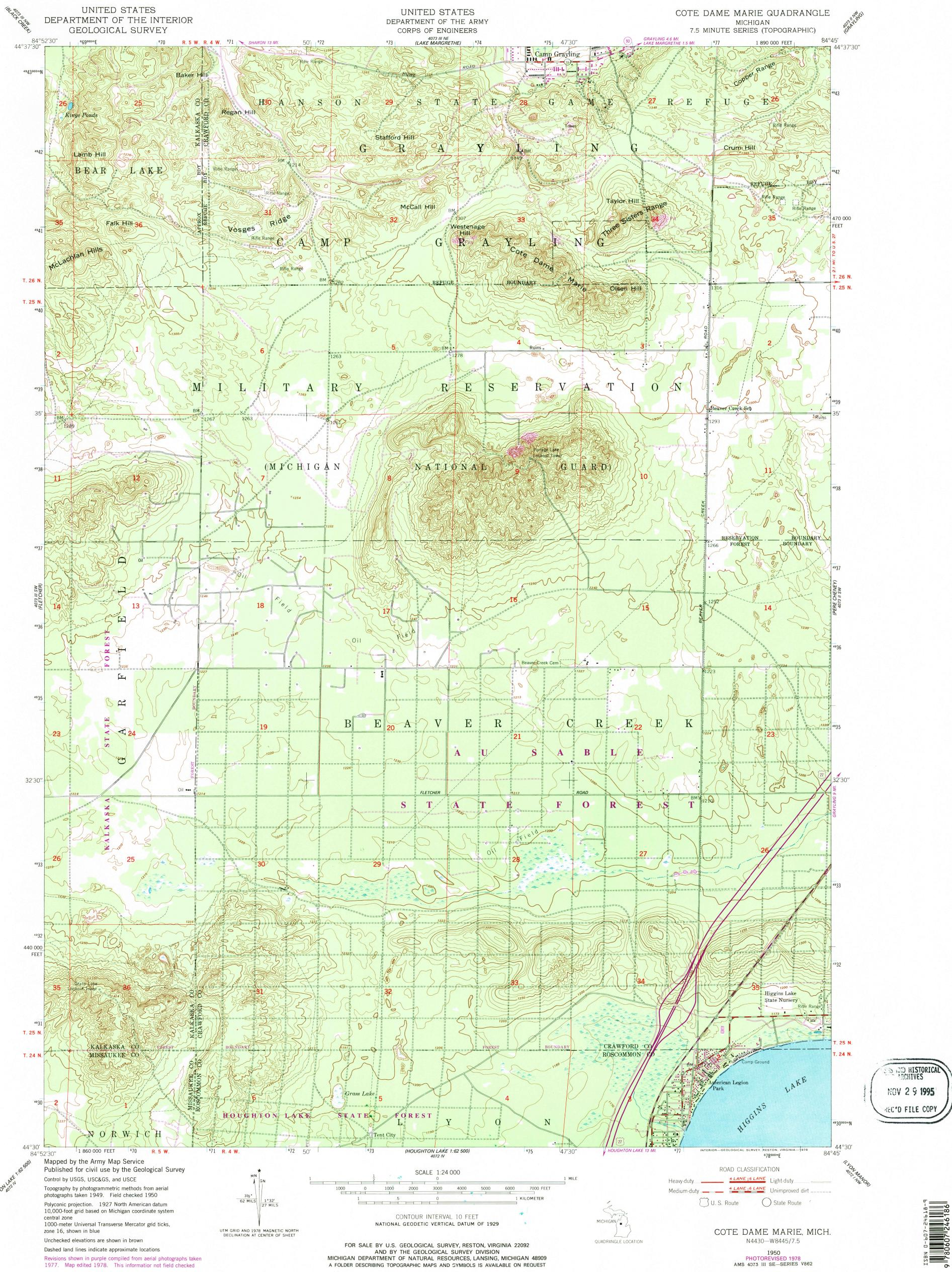
Polyconic projection. 1927 North American datum 10,000-foot grid based on Michigan coordinate system central zone 1000-meter Universal Transverse Mercator grid ticks, UTM GRID AND 1978 MAGNETIC NORTH DECLINATION AT CENTER OF SHEET zone 16, shown in blue Unchecked elevations are shown in brown Dashed land lines indicate approximate locations Revisions shown in purple compiled from aerial photographs taken 1977. Map edited 1978. This informatior not field checked
