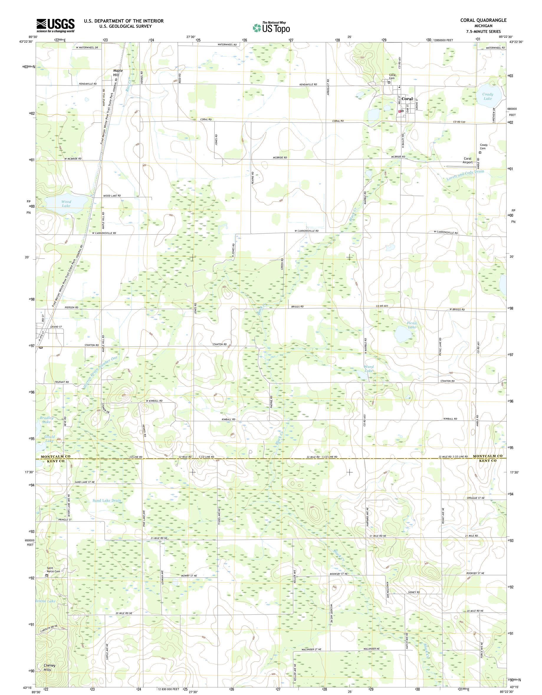
Produced by the United States Geological Survey North American Datum of 1983 (NAD83) World Geodetic System of 1984 (WGS84). Projection and 1 000-meter grid: Universal Transverse Mercator, Zone 16T 10 000-foot ticks: Michigan Coordinate System of 1983 (south zone)
